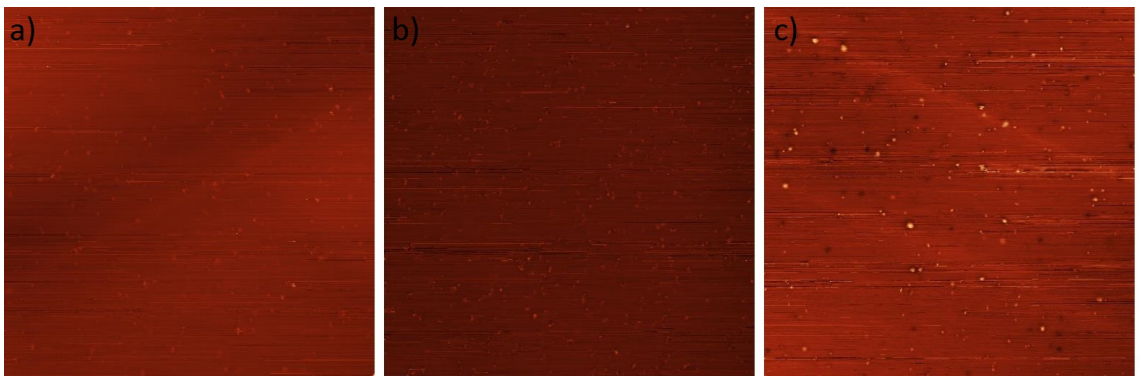
Figure 6.5: 300 nm 2 STM images of Ar + ion irradiated graphite after annealing for 8 hours at (a) 300 °C ( V_{\text{bias}}=1.3 \text{ V} , I=0.8 \text{ nA} ), (b) 500 °C ( V_{\text{bias}}=1.5 \text{ V} , I=0.4 \text{ nA} ) and (c) 750 °C ( V_{\text{bias}}=1.7 \text{ V} , I=0.6 \text{ nA} ).
