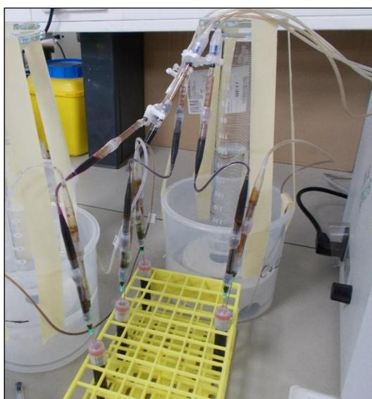
**Figure 3.14** Photograph of backflow of potassium permanganate and water remaining in part of the anaerobic digester set-up at the end of trial 3
