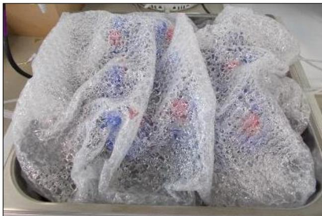
**Figure 2.7** Photograph of the anaerobic digesters insulated in the water bath
