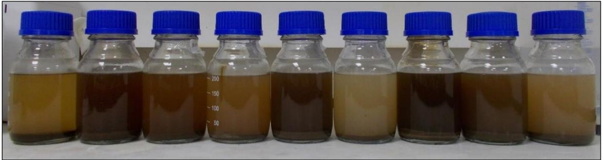
**Figure 3.15** Photograph of anaerobic digester bottles after trial 3. Backflow of potassium permanganate and water during the trial changed colouring. Left to right are control 1, control 2, and control 3, C+LD.A1, C+LD.A2 and C+LD.A3, and C+LD.B1, C+LD.B2 and C+LD.B3
