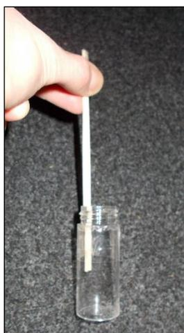
**Figure 2.3** Photograph of the vial on a stick used to sample creamery waste for testing of solids and pH
