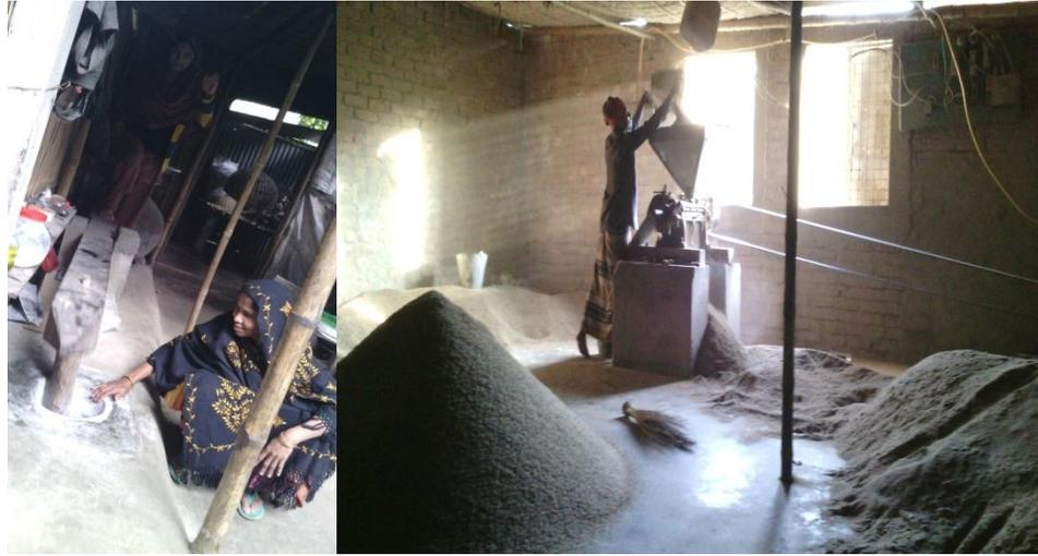
Fig.5.6.3. Rice mills replacing rice husking with *dheki*
