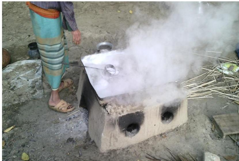
Fig.5.8.2. Specially made *chula* for heating the *khejurer rosh*
