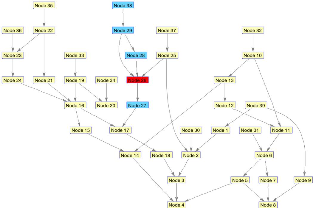
**Figure 5.8:** Tracing example in 39-busbar system with seed node on bus 26 and with threshold value of 1.6 p.u. [29]
