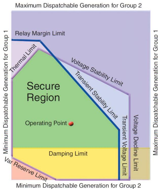
**Figure 3.2:** Security margin nomogram under current OC [44].
