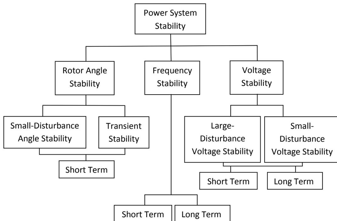
**Figure 3.4:** *Classification of power system stability [43].*
