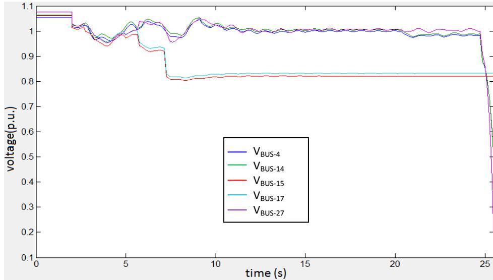
**Figure 6.5:** Voltage drops and collapses during cascading tripping.
