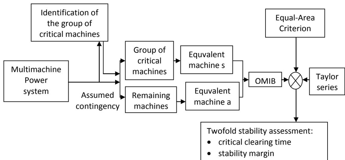
**Figure 7.1:** Principle of the EEAC method [93].
