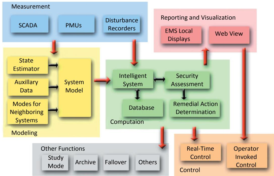
**Figure 3.1:** *Online dynamic security assessment system mechanism [44]*
