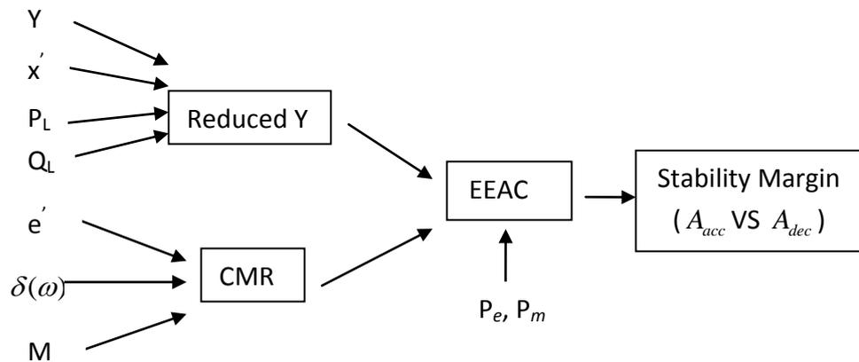
**Figure 7.3:** Measurements needed for calculation in EEAC.
