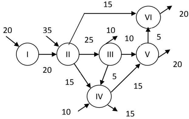
**Figure 5.2:** Tracing example in a 6-busbar network [29].
