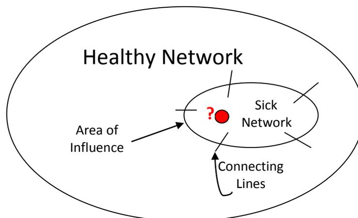
**Figure 5.3:** Tracing method application in controlled islanding [77]
