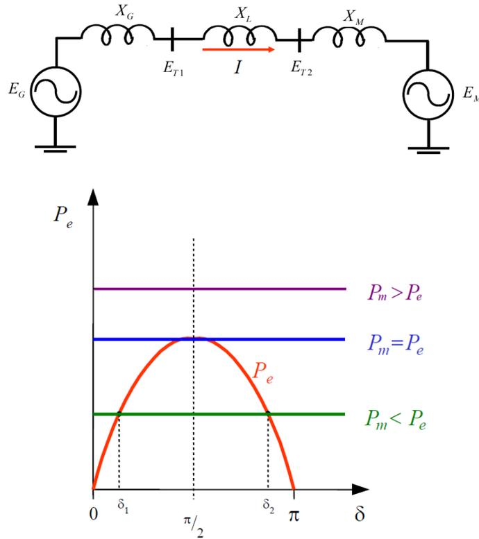
**Figure 3.5:** Idealized model and power-angle curve [63].
