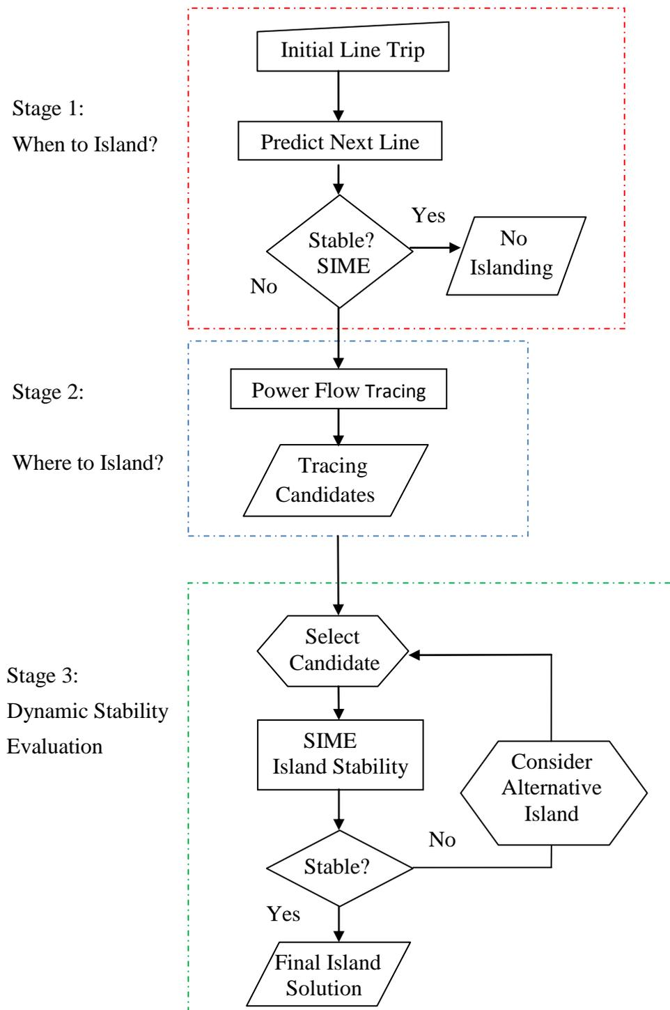
**Figure 8.2:** Flowchart of three-stage strategies for controlled islanding.
