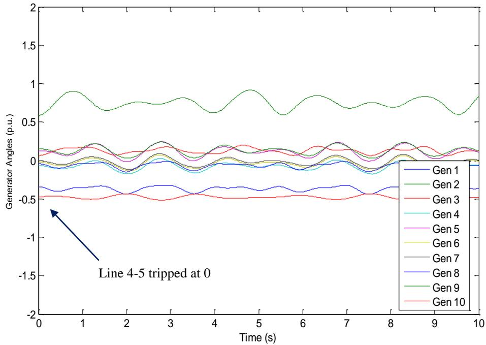
**Figure 9.2:** *Transiently stable case after Line 4-5 was tripped.*
