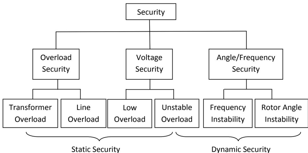
**Figure 3.3:** Categories of the power system's security [61].
