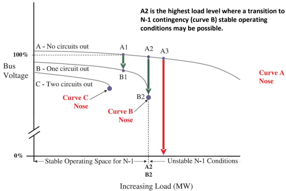
**Figure 2.10:** Real power-voltage ( $P-V$ ) curves [4].
