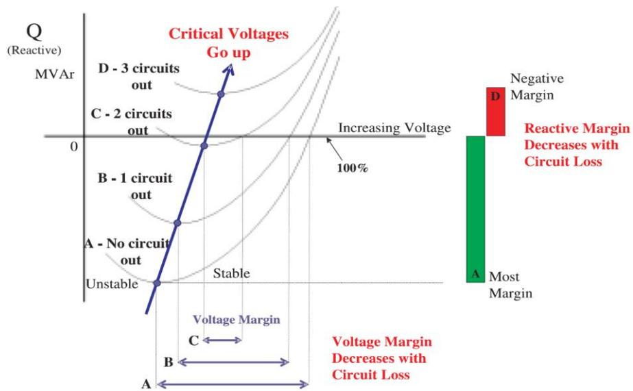
**Figure 2.11:** Reactive power-voltages ( $Q-V$ ) curves [4].
