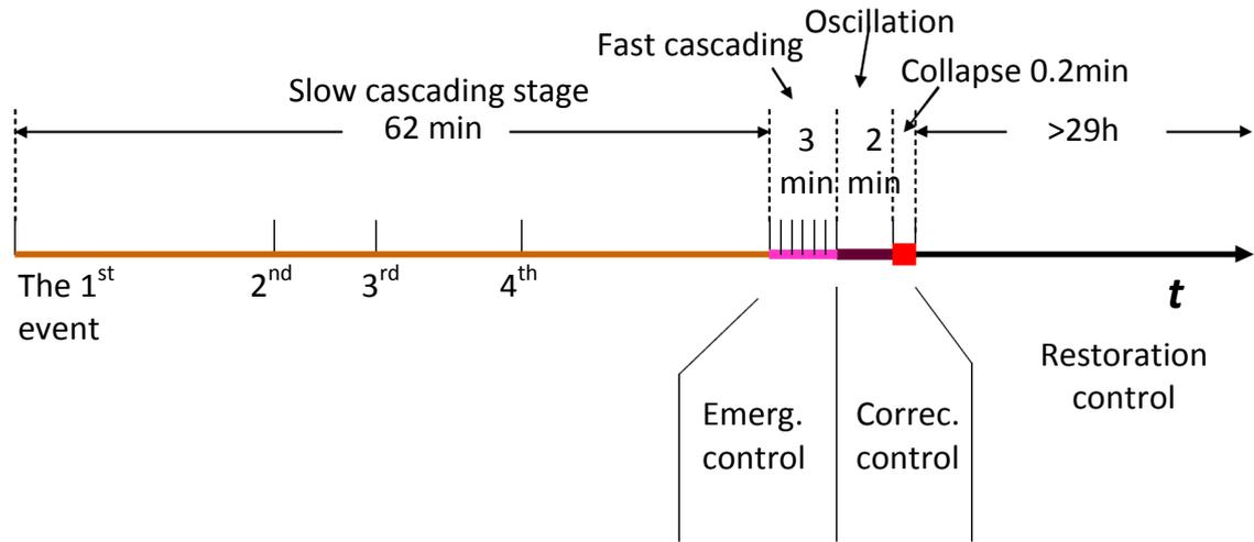
**Figure 2.9:** Typical evolution of US/Canada cascading blackouts [5].
