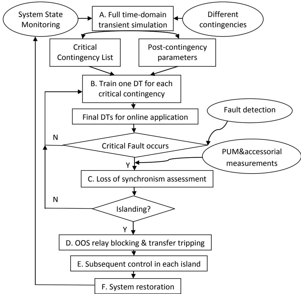
**Figure 4.3:** Proposed DT-based controlled islanding scheme [68].
