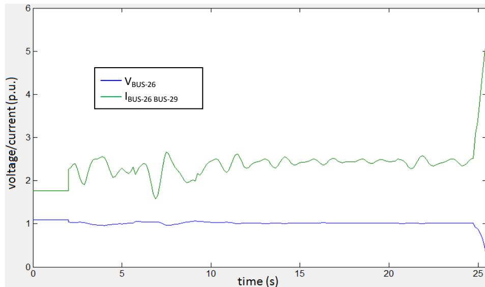
**Figure 6.6:** Line 26-29 is tripped by distance protection.
