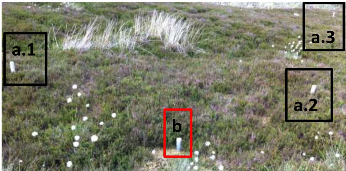
Figure 6.2: An example of a Goyt Valley site triplicate plot (set) (Ravenslow – dry locality, 2013). Visible in the figure are three dipwells (labelled a.1 – a.3) and a 10DD through flow trap (labelled b). Also present in the photo are: three runoff traps, three collars (each plot) and an additional through-flow 10DD trap (between dipwell a.2 and a3), however they are not visible due to the high vegetation.
