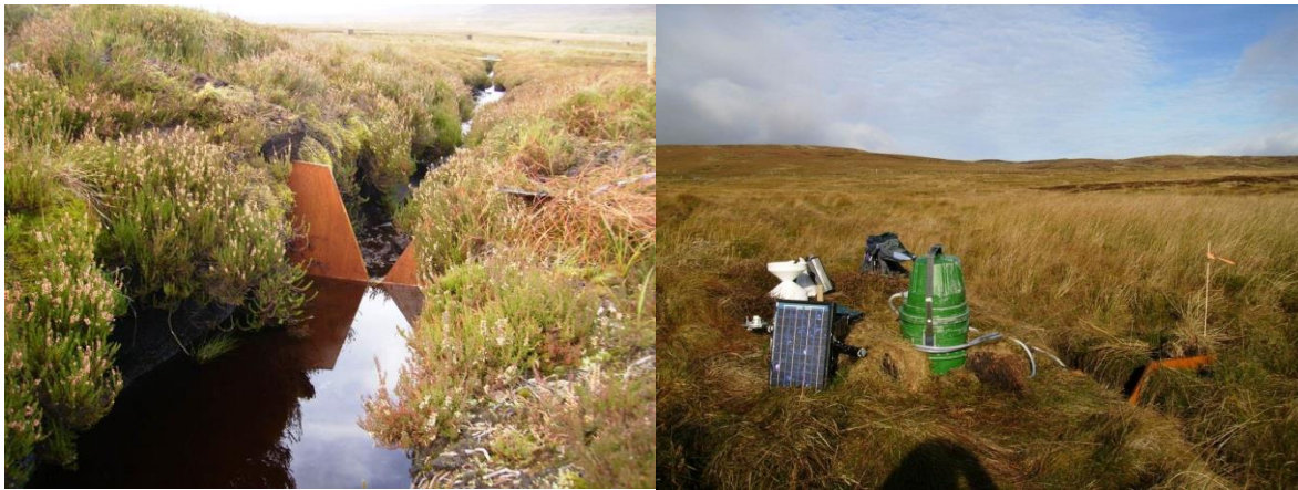
Figure 2.4 Display of V-Notch Weir and Autosampler in Cronkley, 2010.
