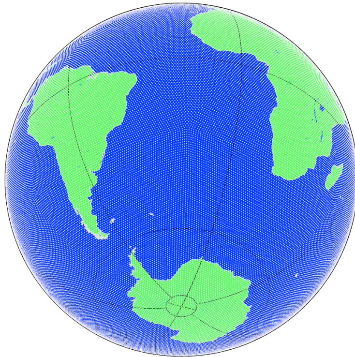
Figure 4.5 – Tegmark pixelisation of the Earth at Tegmark resolution ‘44’, providing 75692 pixels. The Earth is separated into wet (blue) and dry (green) pixels within SELEN.
