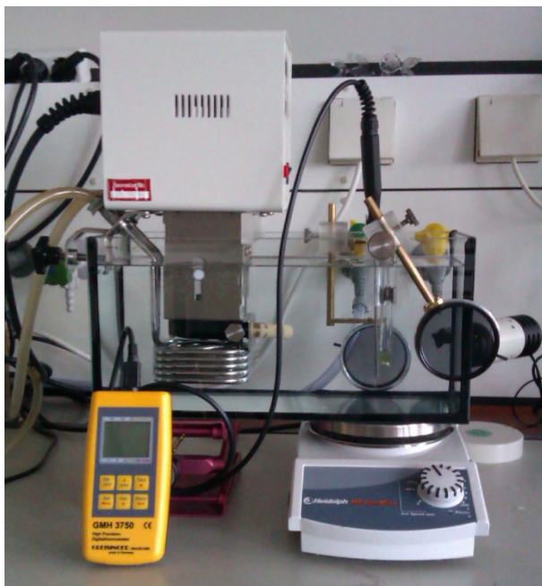
Figure 6.1: Water basin used to determine the phase boundaries of a microemulsion. It is equipped with a thermostat with attached tap water cooling, a magnetic stirrer, a sample holder, a digital thermometer, a lamp and crossed polarisers.
