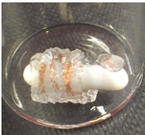
Figure 5: Gel layer surrounding Cu(0) wire.
