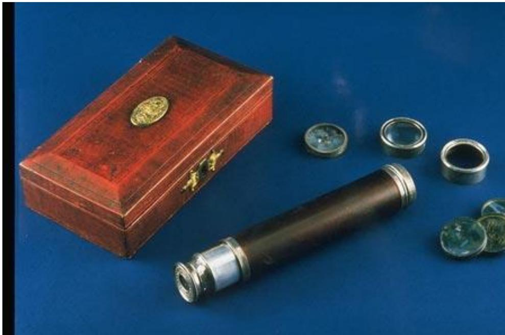
Figure 13. Ruthven’s kaleidoscope, with interchangeable filled glass cells. National Museums Scotland, ref. T.1825.20.
