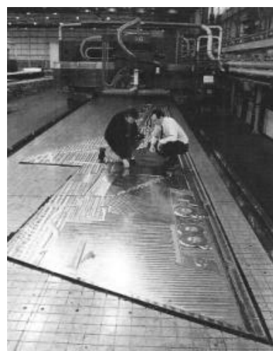
Fig.1.11 Examples of a wing rib (left) and wing skin (right) milled from solid aluminium alloy From Whitford 'Structure and Materials' p.76f
