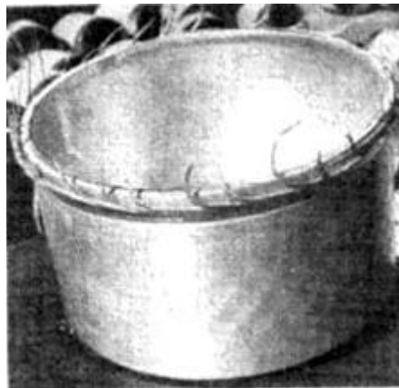
Figure 2.6: Material flaking off a formed part from Nagarajan et al. (1981)
