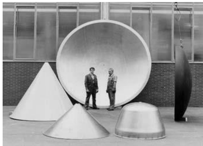
Figure 1.6: 2m diameter parts from Leifield USA (Bewlay, online)
