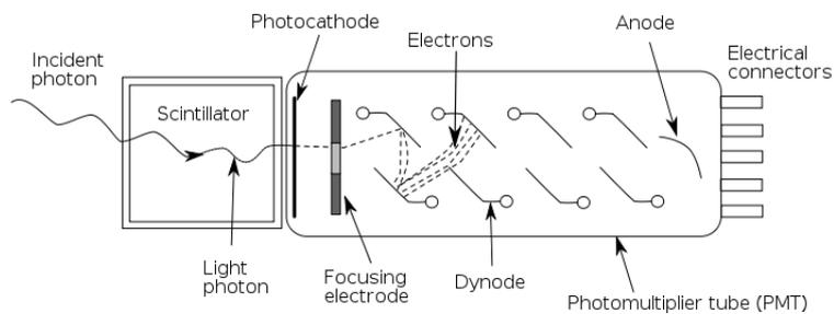
**Figure 18:** Schematic of a basic scintillation detector. The photocathode where the LE photons created from the interaction between the gamma-ray and the crystals are converted into electrons via photoelectric effect can be seen. These photoelectrons then travel through the PMT tube towards the anode and the electrical connectors which record the output information [65].
