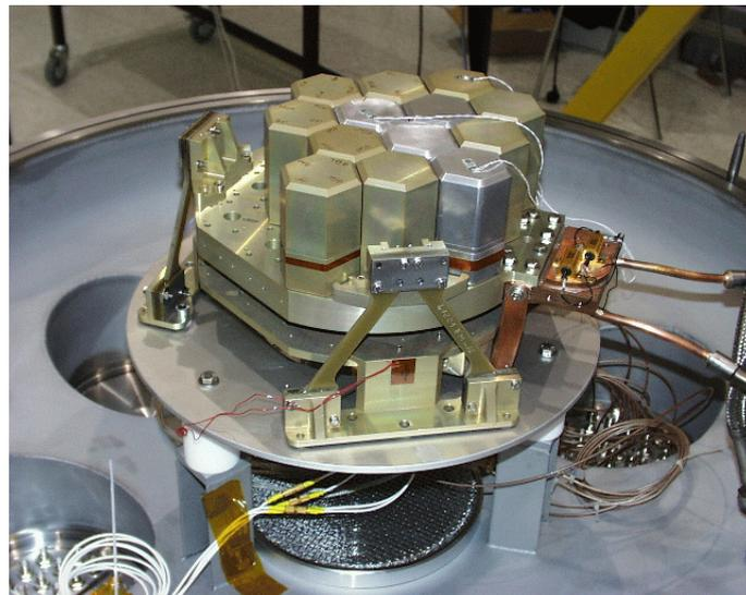
**Figure 21:** Picture of the setup of SPI telescope in the INTEGRAL project. The hexagonal form of the tungsten tiles and the germanium detectors can be clearly seen [67].
