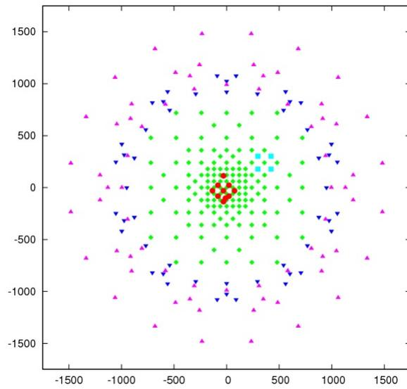
**Figure 38:** Telescope layout for array layout E of PROD1 CTA configuration. Red points are 23m telescopes, black points 12m telescopes, pink points 10m telescopes, green points 6.7m telescopes and blue points 12m telescopes with 10 degrees field-of-view. Credit: Konrad Berlöhr.
