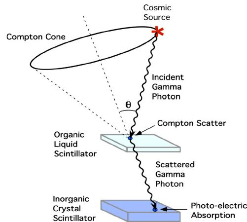
**Figure 22:** Scheme of the basic principle of Compton Scattering Telescopes. Note that the line between the first layer/interaction and the second layer/interaction does not point directly to the initial direction of the incoming gamma-ray. However, the angle of incidence of the photon relative to this line can be determined by applying the Compton scattering law [68].
