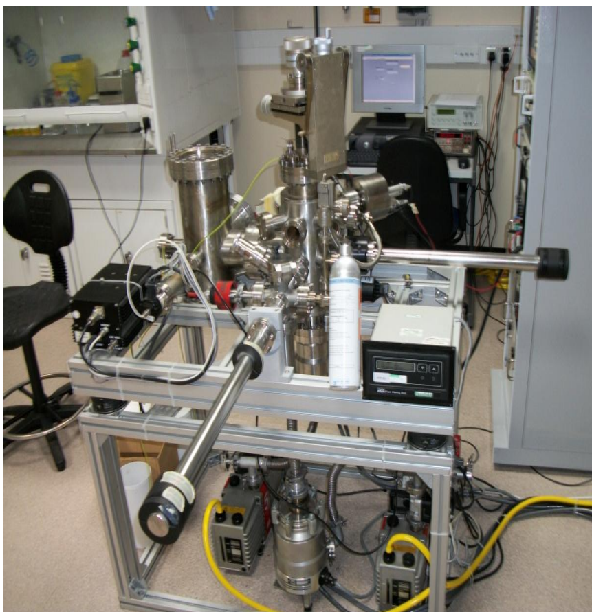
Fig. 3.1: Ultra High Vacuum (UHV) ion gun system at Durham.
