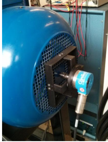
Figure 5-5 Encoder mounted on generator rotor shaft
