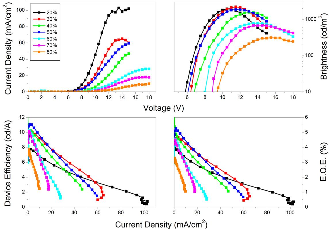
Figure 4.12:  $J$ - $V$ ,  $L$ - $V$  and device efficiency data of single layer devices containing **4.2c** with varying concentrations of OXD-7. Device structure ITO // PEDOT:PSS // PVK:OXD-7:Ir (100:x:8) // Ba (4 nm) // Al (100 nm). Between 30% and 70% OXD-7 there is little variation in peak device efficiency but there is a significant increase in efficiency roll-off and decrease in brightness observed at concentrations of 60% and above.
