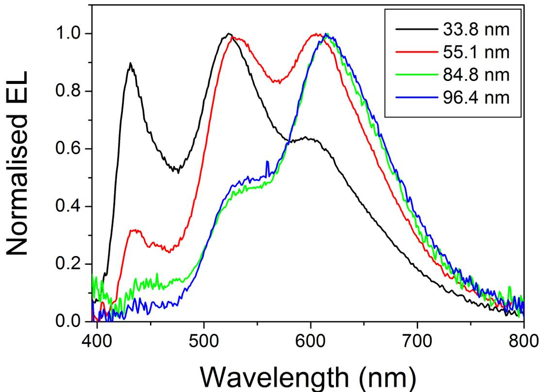
Figure 7.11: Normalised electroluminescence spectra of multilayer devices with varying thicknesses of **7.6**. Device structure ITO // PEDOT:PSS (HIL 1.3) // PVK (30 nm) // **7.6** (x nm) // Ba (4 nm) // Al (62 nm). Again, there is considerable variation in the emission spectrum as the thickness of the emissive layer is changed, with progressively weaker blue/green emission as the layer thickness increases.
