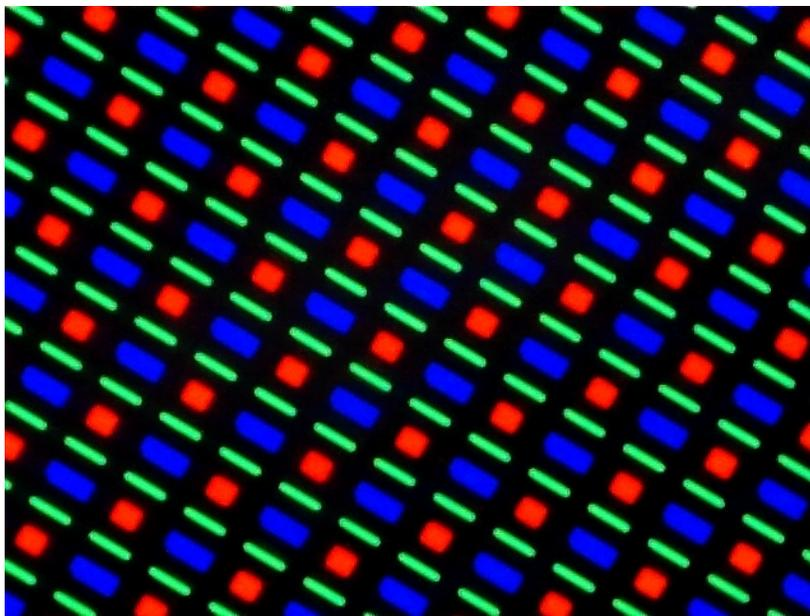
Figure 1.1: Photograph of the Active-Matrix OLED display of a Samsung Galaxy S3 smart phone taken using a Veho VMS-004 USB Microscope at *ca.* 400x magnification showing the PenTile RGBG subpixel matrix. The screen is displaying a plain white background.
