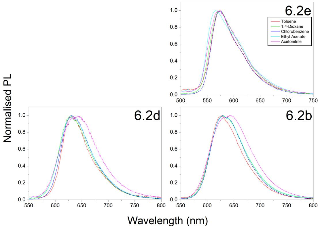
Figure 6.5: Photoluminescence emission spectra of complexes **6.2b**, **6.2d** and **6.2e** in five solvents of increasing polarity: toluene (0.36 D), 1,4-dioxane (0.45 D), chlorobenzene (1.54 D), ethyl acetate (1.88 D) and acetonitrile (3.84 D) [17], demonstrating the weaker solvatochromic effect exhibited by series **6.2** complexes.
