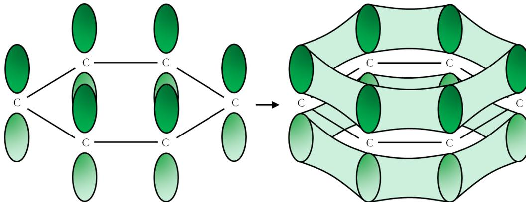
Figure 2.4: Representation of the formation of delocalised  $\pi$  molecular orbitals in a benzene ring, an example of a conjugated system. Bonds to hydrogen atoms are not shown, while  $\sigma$  bonds between carbon atoms are represented as a straight line. Conjugation leads to overlap of the six out of plane p orbitals (left) to form regions of delocalised electron density above and below the plane of the molecule (right).
