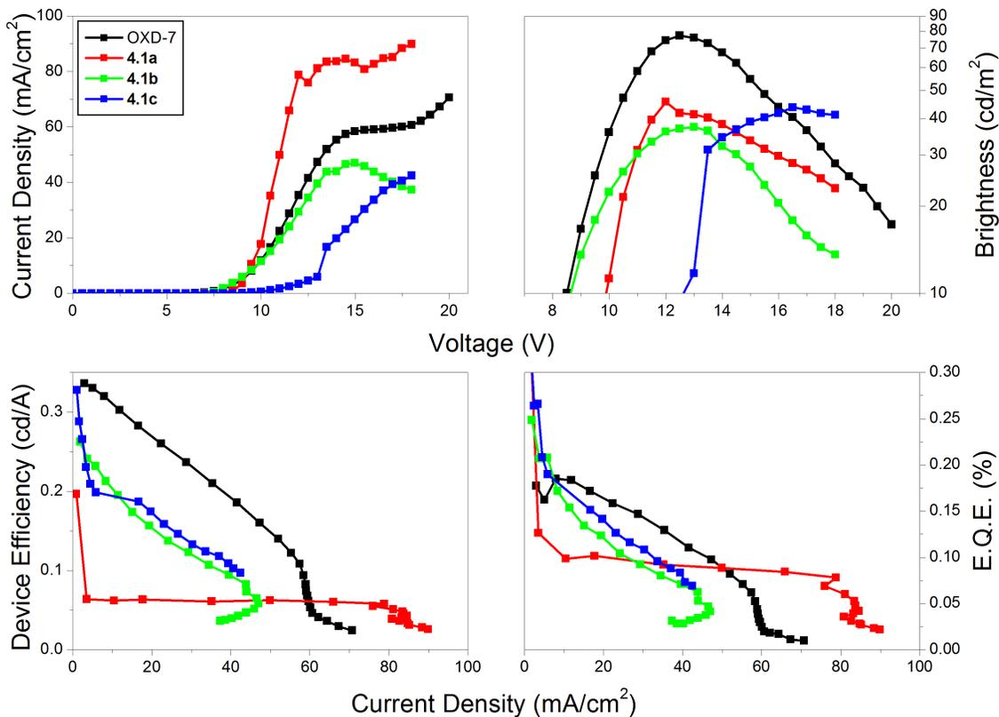
Figure 4.4:  $J$ - $V$ ,  $L$ - $V$  and device efficiency data of single layer devices consisting of PVK blended with each electron transport material without any dopant emitter. Device structure ITO // PEDOT:PSS // PVKL:ET (100:30) (*ca.* 80 nm) // Ba (4 nm) // Al (100 nm).
