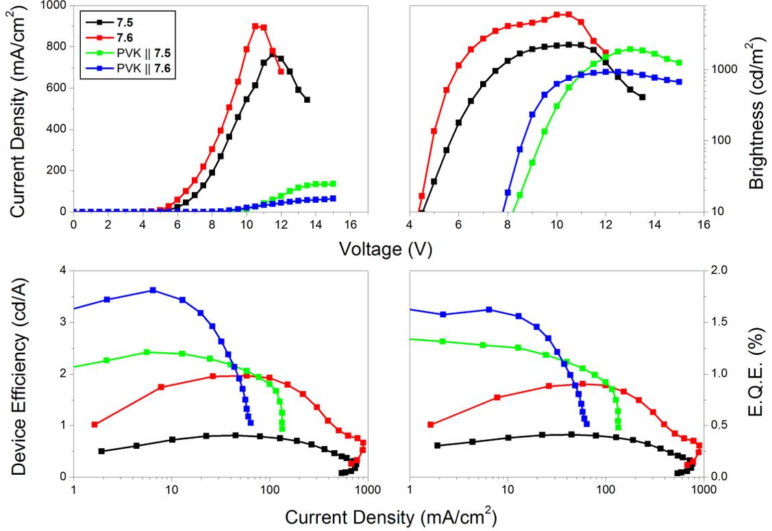
Figure 7.13:  $J$ - $V$ ,  $L$ - $V$  and device efficiency data for single layer and multilayer devices comparing **7.5** and **7.6**. Device structure ITO // PEDOT:PSS (HIL 1.3) // PVK (30 nm) (multilayer devices only) // **7.5** or **7.6** // Ba (4 nm) // Al (100 nm).
