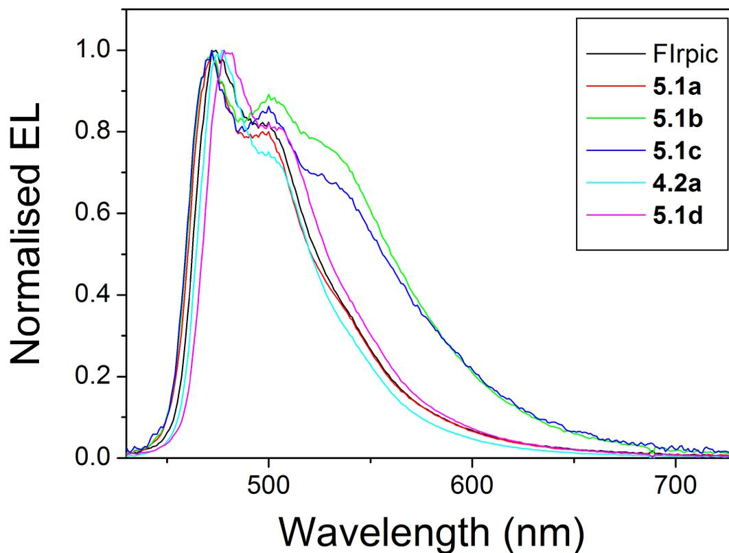
Figure 5.5: Normalised electroluminescence spectra of the blue iridium emitters **5.1a-d**, **4.2a** and FIrpic in single layer devices. The CIE coordinates at 12 V are as follows: FIrpic - (0.17, 0.38), **5.1a** - (0.17, 0.36), **5.1b** - (0.24, 0.43), **5.1c** - (0.24, 0.41), **4.2a** - (0.16, 0.38), **5.1d** - (0.18, 0.43).
