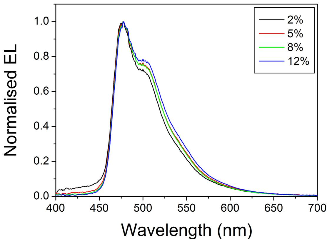
Figure 4.16: Normalised electroluminescence spectra of single layer devices containing **4.2c** at varying concentrations. Device structure ITO // PEDOT:PSS // PVK:OXD-7:Ir (100:50:x) // Ba (4 nm) // Al (100 nm). Increasing iridium emitter concentration again increases the relative intensity of the shoulder in the emission spectrum, although this could also be due to an increase in the layer thickness.
