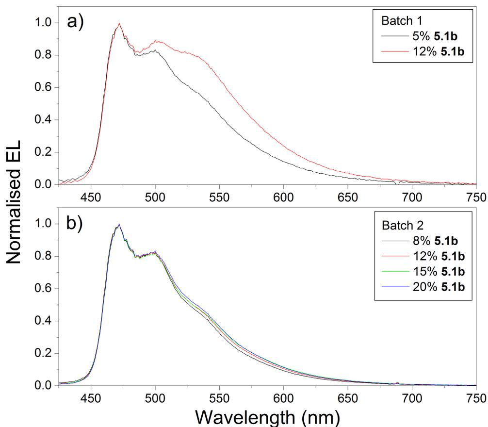
Figure 5.7: Normalised electroluminescence spectra of **5.1b** showing the concentration dependence of emission using two different batches of the same material in single layer devices. The second batch, shown in panel (b), does not exhibit the broad green shoulder that was observed in initial measurements of the first batch, shown in panel (a).
