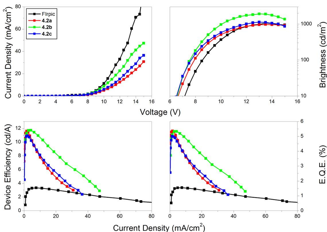
Figure 4.17:  $J$ - $V$ ,  $L$ - $V$  and device efficiency data of single layer devices comparing complexes **4.2a-c** with FIrpic. Device structure ITO // PEDOT:PSS // PVK:OXD-7:Ir (100:50:12, 78 nm) // Ba (4 nm) // Al (60 nm). All new complexes exhibit comparable maximum efficiencies, significantly outperforming FIrpic. However less efficiency roll off is observed for complex **4.2c**.
