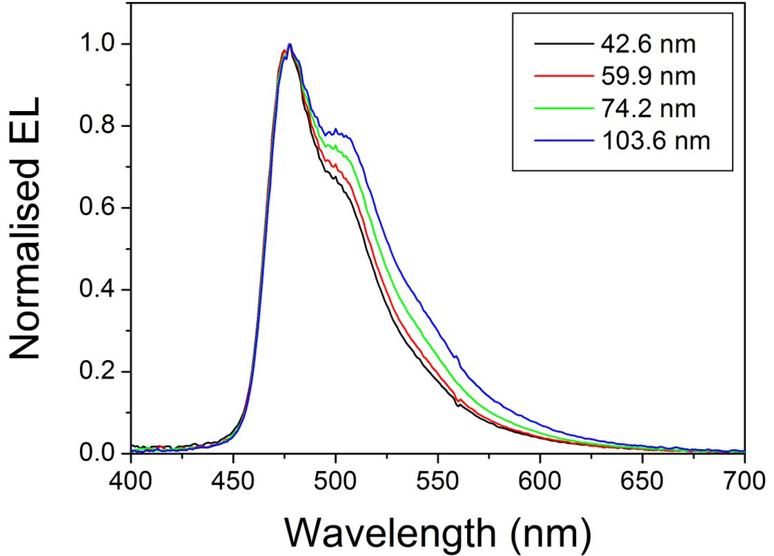
Figure 4.11: Normalised electroluminescence spectra of single layer devices containing **4.2c** with varying layer thickness. Device structure ITO // PEDOT:PSS // PVK:OXD-7:Ir (100:40:8) // Ba (4 nm) // Al (79 nm). Increasing layer thickness increases the relative intensity of the shoulder in the emission spectrum.
