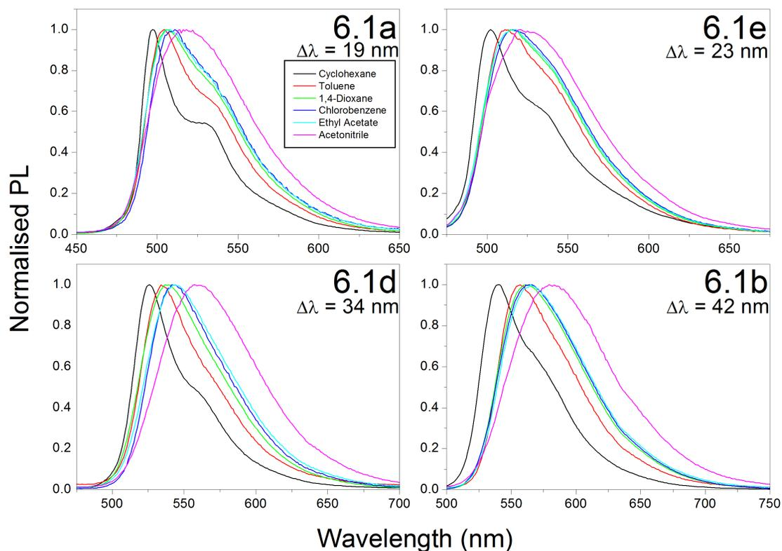
Figure 6.4: Photoluminescence emission spectra of complexes **6.1a**, **6.1b**, **6.1d** and **6.1e** in six solvents of increasing polarity: cyclohexane (non-polar), toluene (0.36 D), 1,4-dioxane (0.45 D), chlorobenzene (1.54 D), ethyl acetate (1.88 D) and acetonitrile (3.84 D) [17], demonstrating the increasing solvatochromic shift  $\Delta\lambda$  observed as the molecular dipole moment of the complex increases.
