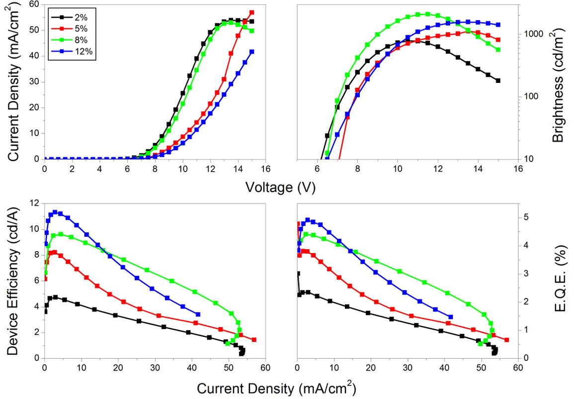
Figure 4.15:  $J$ - $V$ ,  $L$ - $V$  and device efficiency data of single layer devices containing **4.2c** at varying concentrations. Device structure ITO // PEDOT:PSS // PVK:OXD-7:Ir (100:50:x) // Ba (4 nm) // Al (100 nm). The efficiency of devices increases as the emitter concentration increases, but at the highest concentration a larger efficiency roll-off is observed.
