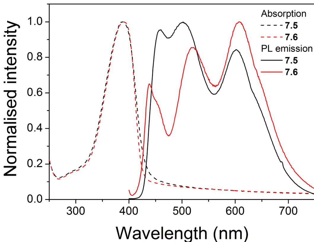
Figure 7.5: Comparison of the normalised absorption and photoluminescence emission spectra of copolymer **7.6**, not containing the S unit, with the S-containing copolymer **7.5** in film. The excitation wavelength for the PL emission measurement was 390 nm.
