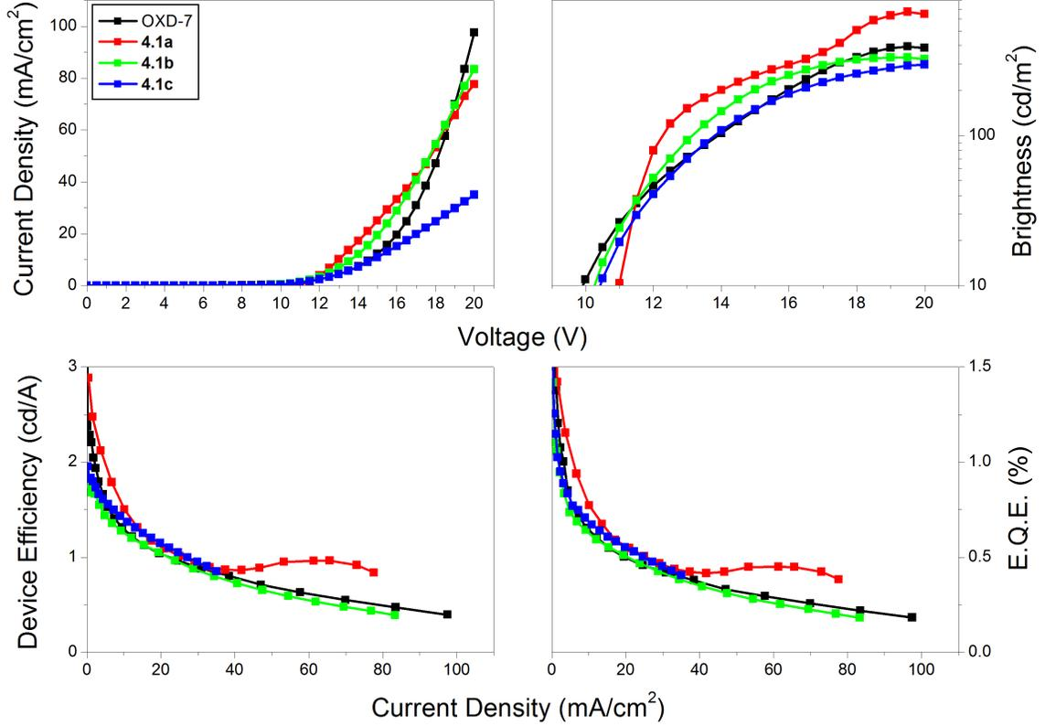
Figure 4.2:  $J$ - $V$ ,  $L$ - $V$  and device efficiency data of multilayer devices consisting of PVK blended with each electron transport material and FIrpc. ITO // PEDOT:PSS // PVKH (20 nm) // PVKL:ET:FIrpc (100:30:2) (*ca.* 81 nm) // Ba (4 nm) // Al (100 nm).
