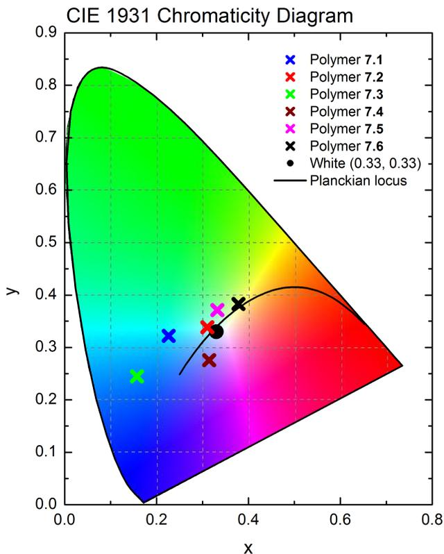
Figure 7.6: CIE chromaticity diagram showing the coordinates of photoluminescence emission for polymers **7.1** to **7.6**. Polymers **7.2** (0.31, 0.34), **7.5** (0.33, 0.37) and **7.6** (0.38, 0.38) in particular show promising emission for white OLED devices.
