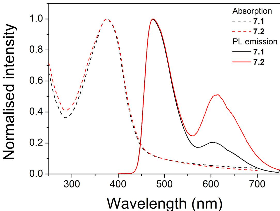
Figure 7.3: Normalised absorption and photoluminescence emission spectra of the two carbazole-based white-emitting copolymers **7.1** and **7.2** in film. The excitation wavelength for the PL emission measurement was 375 nm.
