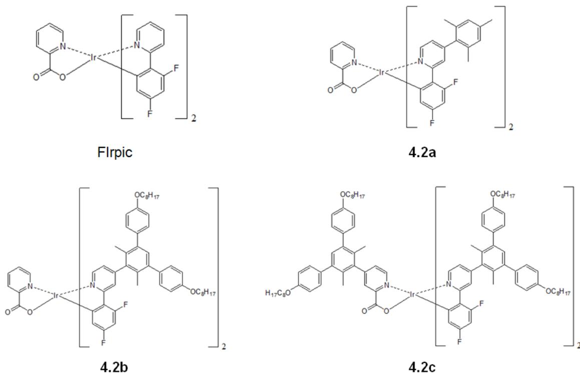
Figure 4.7: Chemical structures of the blue emitting iridium complexes **4.2a-c** characterised in this section as well as that of FIrpic. These aim to improve the solubility of FIrpic and, in the case of **4.2b-c**, shield the iridium core by functionalisation of the ligands with bulky aryl side chains.
