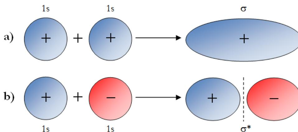
Figure 2.3: Representation of the formation of bonding and antibonding  $\sigma$  and  $\sigma^*$  molecular orbitals by the overlap of s orbitals. In phase addition (a) results in formation of a bonding  $\sigma$  molecular orbital, while out of phase addition (b) results in formation of a higher energy  $\sigma^*$  antibonding molecular orbital.
