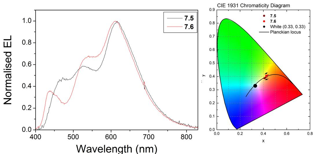
Figure 7.18: Left: Normalised electroluminescence spectra of multilayer devices comparing **7.5** and **7.6** incorporating an electron transporting layer of TPBI. Device structure ITO // PEDOT:PSS (HIL 1.5) // PVK (30 nm) // **7.5** or **7.6** // TPBI (30 nm) // LiF (1 nm) // Al (100 nm). Right: CIE chromaticity diagram showing the CIE coordinates of the devices, also indicating the extent and direction of the colour shift with increasing voltage.
