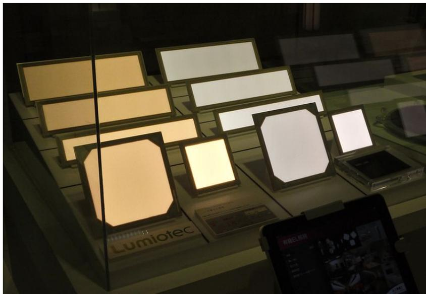
Figure 1.3: Photograph of a selection of OLED lighting demonstration panels produced by Lumiotech [26].
