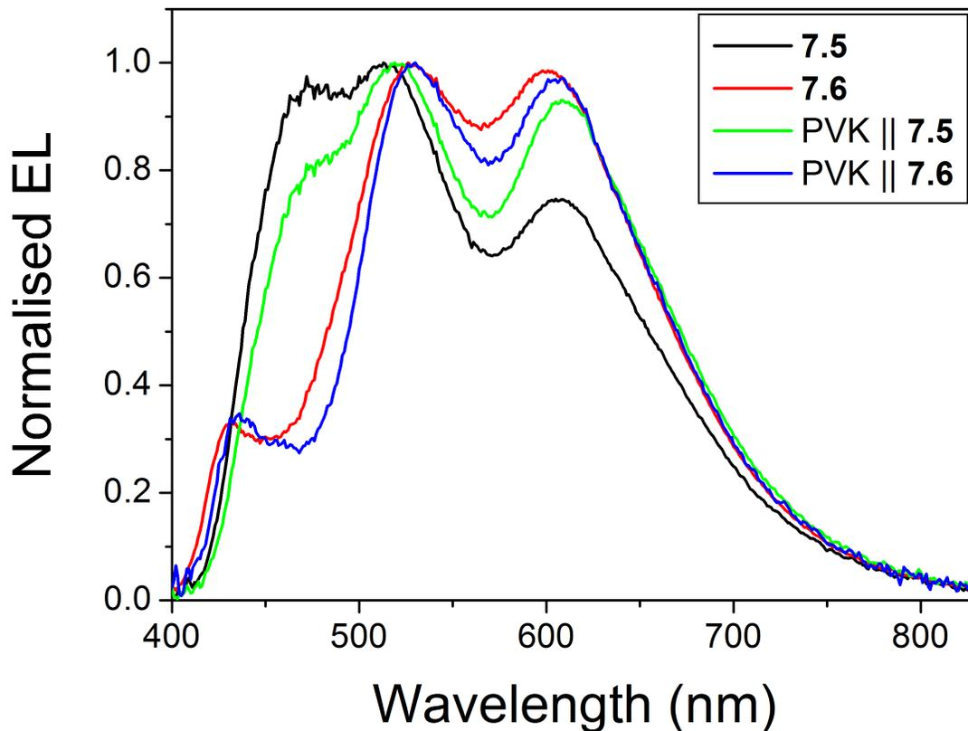
Figure 7.14: Normalised electroluminescence spectra of single layer and multilayer devices comparing **7.5** and **7.6**. Device structure ITO // PEDOT:PSS (HIL 1.3) // PVK (30 nm) (multilayer devices only) // **7.5** or **7.6** // Ba (4 nm) // Al (100 nm).
