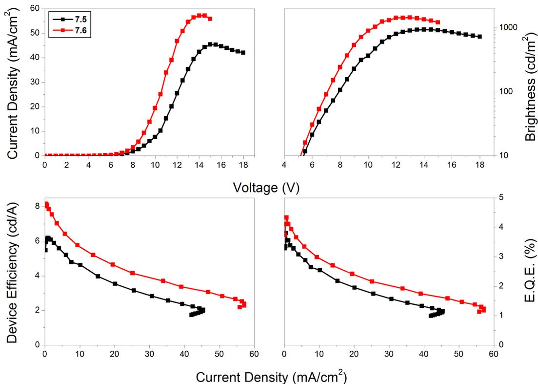
Figure 7.17:  $J$ - $V$ ,  $L$ - $V$  and device efficiency data for multilayer devices comparing **7.5** and **7.6** incorporating an electron transporting layer of TPBI. Device structure ITO // PEDOT:PSS (HIL 1.5) // PVK (30 nm) // **7.5** or **7.6** // TPBI (30 nm) // LiF (1 nm) // Al (100 nm).
