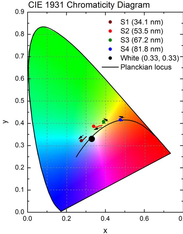
Figure 7.9: CIE chromaticity diagram showing coordinates of the electroluminescence of polymer **7.5** at different thicknesses, also indicating the extent and direction of the colour shift with increasing voltage. Device structure ITO // PEDOT:PSS (HIL 1.1) // PVK (30 nm) // **7.5** (x nm) // Ba (4 nm) // Al (125 nm). The emission shifts progressively away from the white point with increasing thickness. Coordinates:
