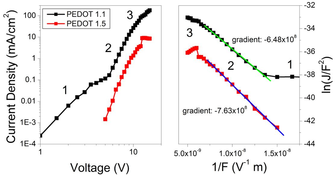
Figure 5.20: Left: log-log plot of the  $J$ - $V$  data from devices with different PEDOT:PSS hole injection layer. Right: Fowler-Nordheim plot of the same data showing the gradient of the hole injection region.
