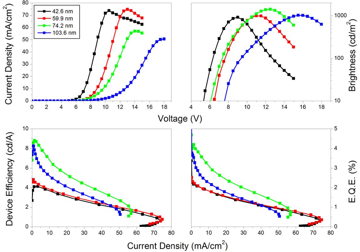
Figure 4.10:  $J$ - $V$ ,  $L$ - $V$  and device efficiency data of single layer devices containing **4.2c** with varying layer thickness. Device structure ITO // PEDOT:PSS // PVK:OXD-7:Ir (100:40:8) // Ba (4 nm) // Al (79 nm). Increasing emissive layer thickness generally increases the turn on voltage, and the highest device efficiency was achieved with an emissive layer thickness of 74.2 nm.
