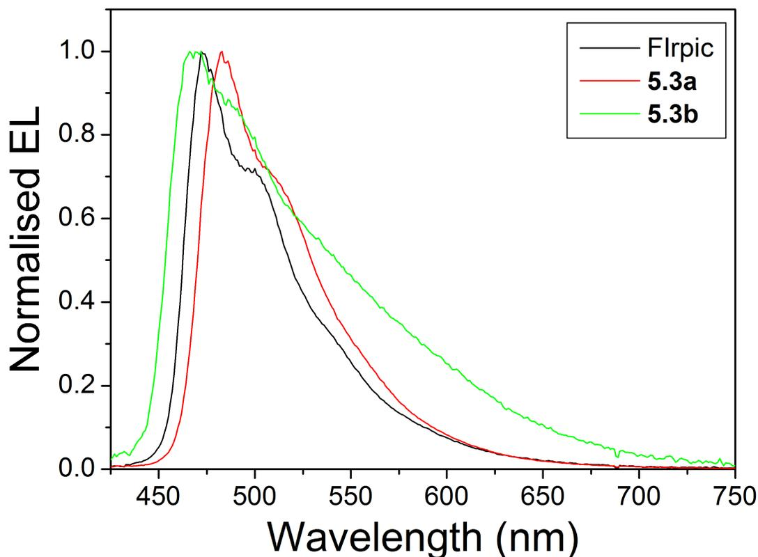
Figure 5.18: Normalised electroluminescence spectra of the carbazole-based iridium emitters **5.3a-b** compared with FIrpic and complex **4.2a**. Device structure ITO // PEDOT:PSS (HIL 1.5) // PVK:OXD-7:Ir (100:50:8) // TPBI (25 nm) // LiF (1 nm) // Al (100 nm)
