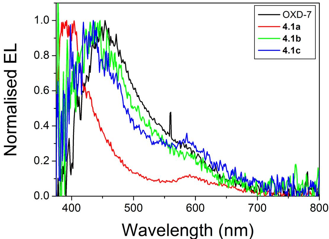
Figure 4.5: Normalised electroluminescence spectra of single layer devices consisting of PVK blended with each electron transport material, showing the exciplex emission observed from **4.1b-c** and OXD-7. The emission from the **4.1a** device is that of PVK.
