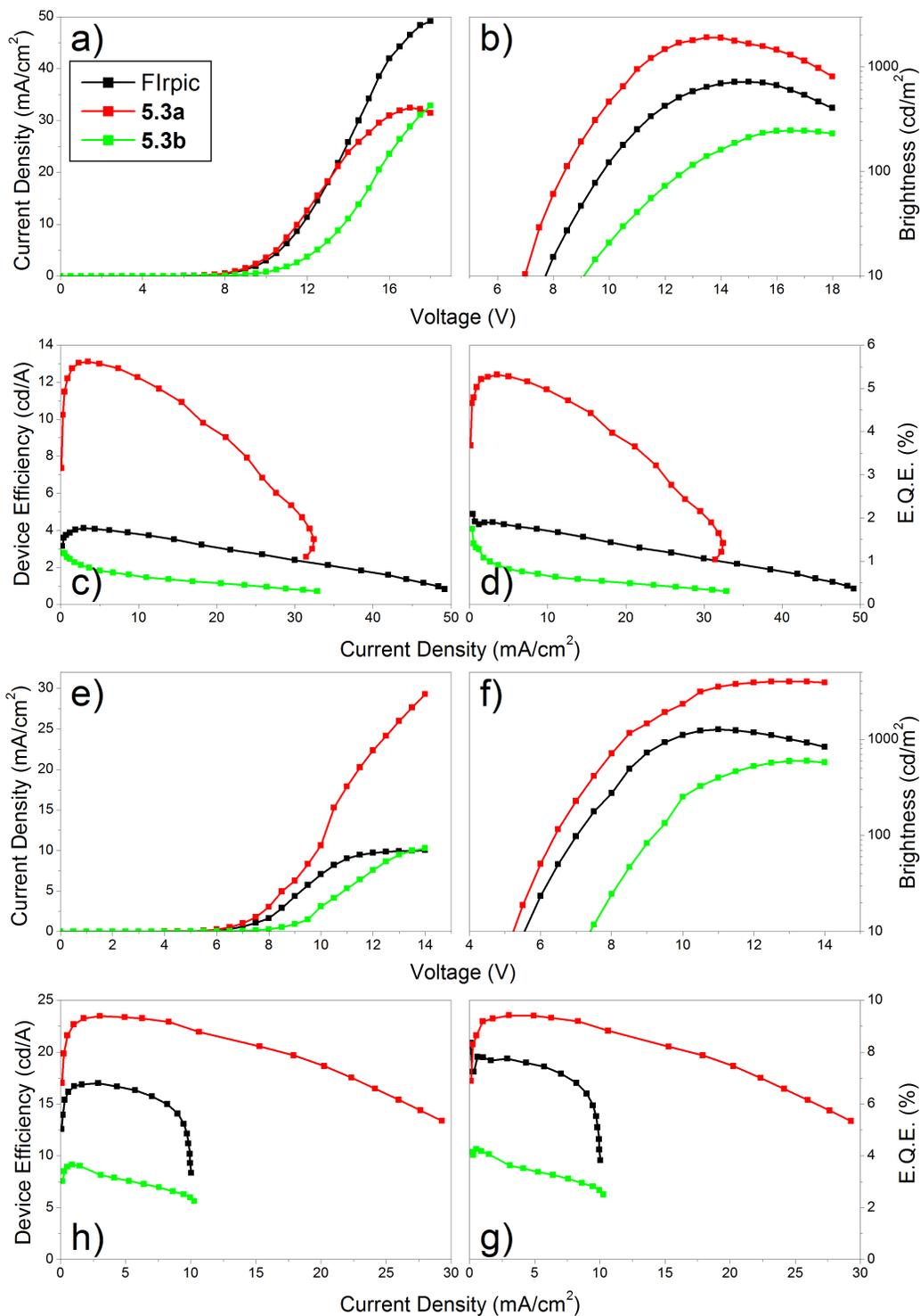
Figure 5.17:  $J$ - $V$ ,  $L$ - $V$  and device efficiency data comparing **5.3a-b** and FIrpic for (panels a - d) single layer devices with structure ITO // PEDOT:PSS (HIL 1.5) // PVK:OXD-7:Ir (100:50:12, 78 nm) // Ba (4 nm) // Al (80 nm), and (panels e - h) bilayer devices with structure ITO // PEDOT:PSS (HIL 1.5) // PVK:OXD-7:Ir (100:50:8) // TPBI (25 nm) // LiF (1 nm) // Al (100 nm).
