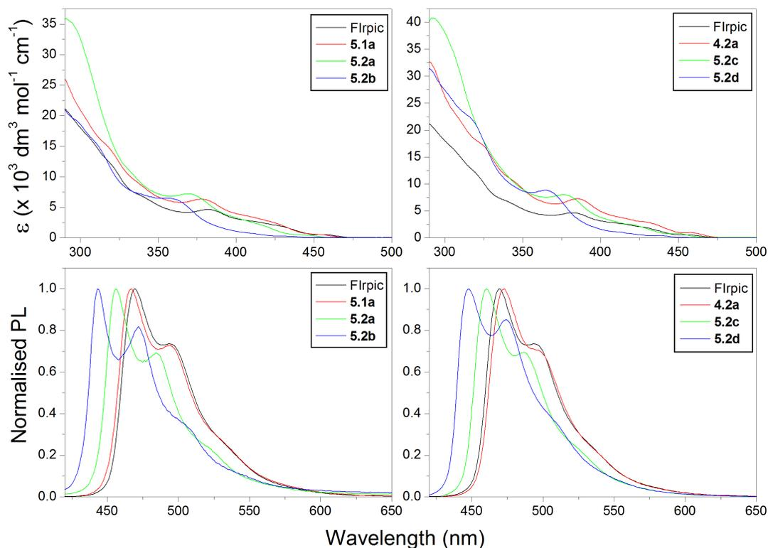
Figure 5.9: Extinction coefficient spectra (top) and normalised photoluminescence spectra (bottom) in toluene solution of (left) the blueshifted iridium emitters **5.2a-b** compared to the parent complex **5.1a** and FIrpc, and (right) **5.2c-d** compared to the parent complex **4.2a** and FIrpc. The excitation wavelength for PL measurements was 400 nm.
