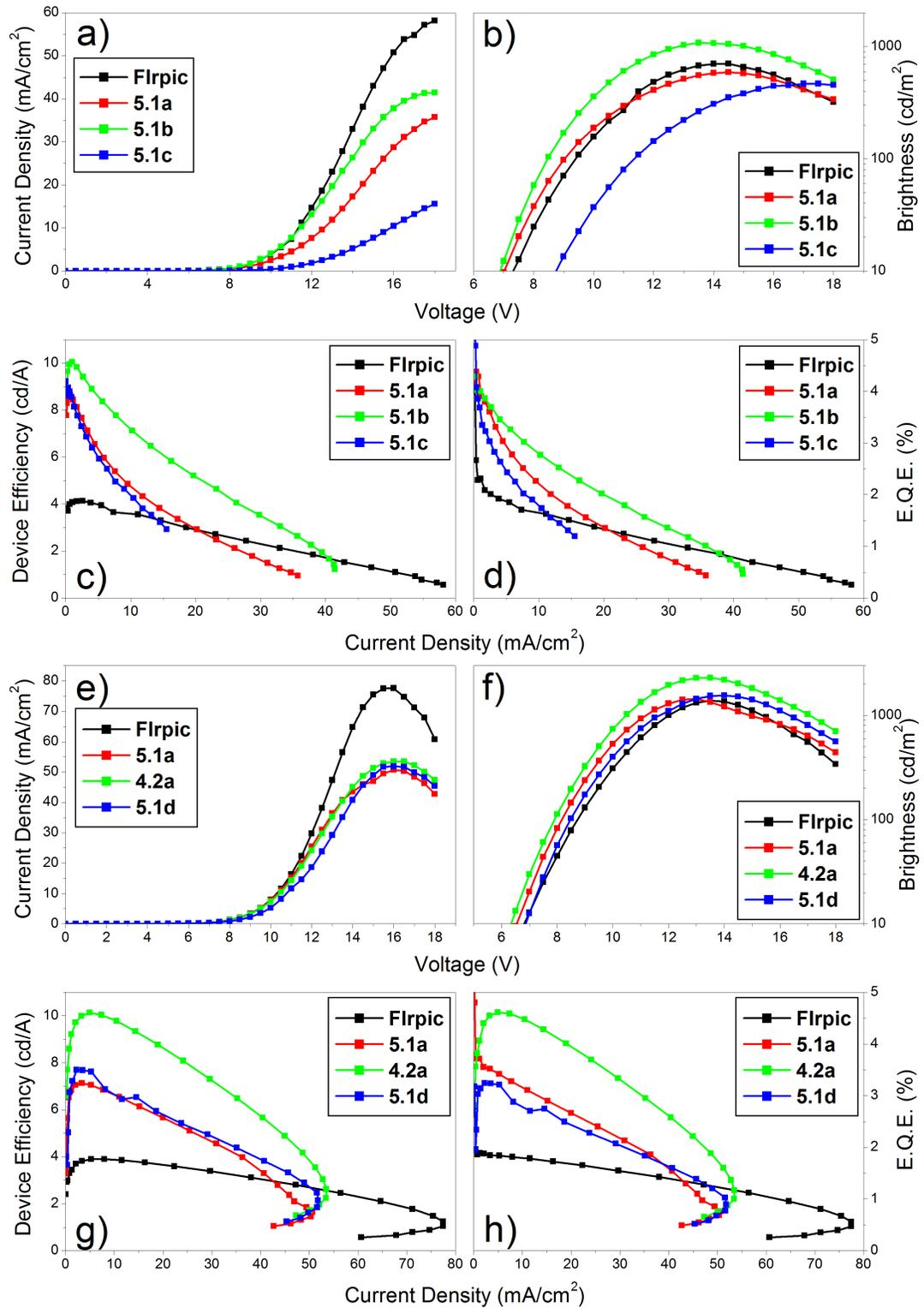
Figure 5.6:  $J$ - $V$ ,  $L$ - $V$  and device efficiency data for single layer devices comparing (panels a - d) Flrpic and 5.1a-c and (panels e - h) Flrpic and 5.1a, 4.2a and 5.1d. Device structure ITO // PEDOT:PSS (HIL 1.5) // PVK:OXD-7:Ir (100:50:12, 76 nm) // Ba (4 nm) // Al (100 nm).
