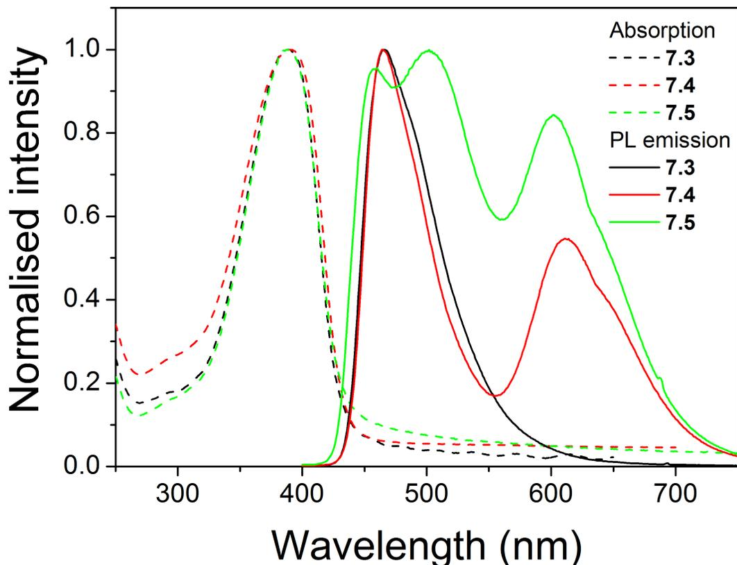
Figure 7.4: Normalised absorption and photoluminescence emission spectra of the three arylamine-based copolymers **7.3**, **7.4** and **7.5** in film. The excitation wavelength for the PL emission measurement was 390 nm.
