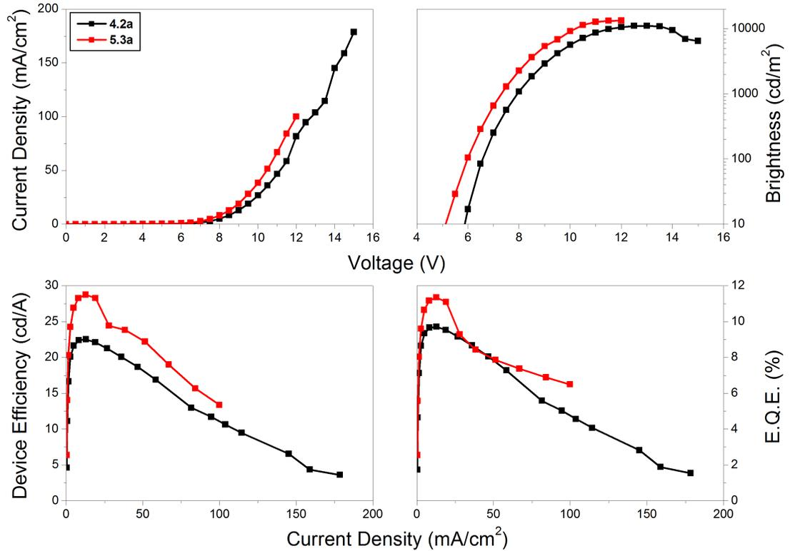
Figure 5.19:  $J$ - $V$ ,  $L$ - $V$  and device efficiency data comparing **5.3a** with **4.2a** in bilayer devices with structure ITO // PEDOT:PSS (HIL 1.1) // PVK:OXD-7:Ir (100:50:8) // TPBI (32 nm) // LiF (0.7 nm) // Al (100 nm).
