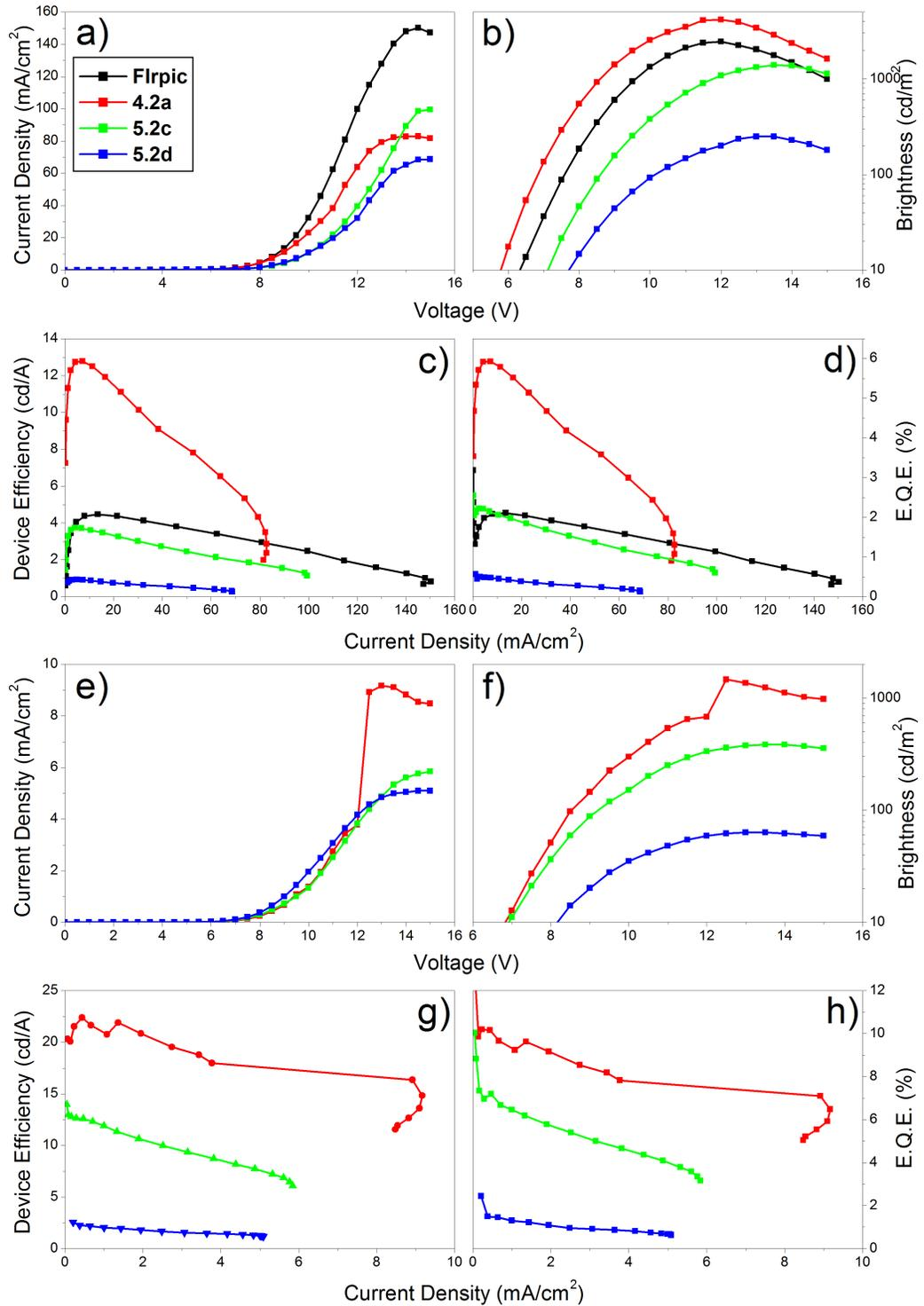
Figure 5.11:  $J$ - $V$ ,  $L$ - $V$  and device efficiency data comparing **5.2c-d** and **4.2a** for (panels a - d) single layer devices (also compared to Flrpic) with structure ITO // PEDOT:PSS (HIL 1.1) // PVK:OXD-7:Ir (100:50:12, 75 nm) // Ba (4 nm) // Al (80 nm), and (panels e - h) bilayer devices with structure ITO // PEDOT:PSS (HIL 1.5) // PVK:OXD-7:Ir (100:50:8) // TPBI (32 nm) // LiF (0.7 nm) // Al (100 nm).
