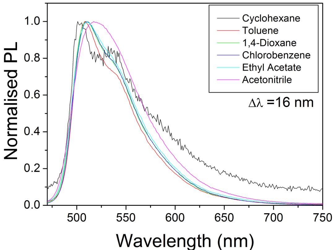
Figure 6.6: Solvatochromic shift in the emission spectrum of Ir(ppy)<sub>3</sub> in six solvents of increasing polarity, for comparison with series **6.1** complexes. A shift of 16 nm is observed, compared to 19 nm for the parent complex **6.1a**.
