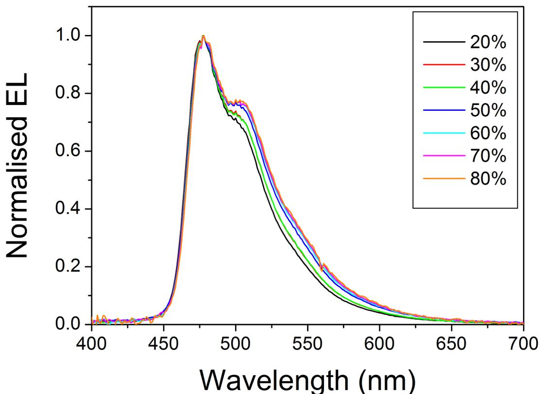
Figure 4.14: Normalised electroluminescence spectra of single layer devices containing **4.2c** with varying concentrations of OXD-7. Device structure ITO // PEDOT:PSS // PVK:OXD-7:Ir (100:x:8) // Ba (4 nm) // Al (100 nm). Increasing OXD-7 concentration increases the relative intensity of the shoulder in the emission spectrum, although this could also be due to an increase in the layer thickness.
