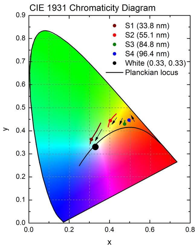
Figure 7.12: CIE chromaticity diagram showing coordinates of the electroluminescence of polymer **7.6** at different thicknesses, also indicating the extent and direction of the colour shift with increasing voltage. Device structure ITO // PEDOT:PSS (HIL 1.3) // PVK (30 nm) // **7.6** (x nm) // Ba (4 nm) // Al (62 nm). The emission shifts progressively away from the white point with increasing thickness.
