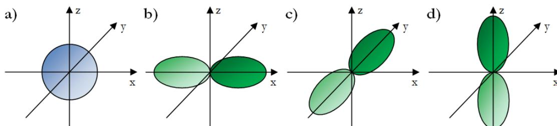
Figure 2.1: Schematic of s and p atomic orbitals, where the atom is located at the origin of the coordinate system. The s orbital is shown in a), while the degenerate  $p_x$ ,  $p_y$  and  $p_z$  orbitals are represented in b), c) and d) respectively.
