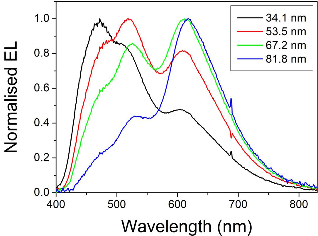
Figure 7.8: Normalised electroluminescence spectra of multilayer devices with varying thicknesses of **7.5**. Device structure ITO // PEDOT:PSS (HIL 1.1) // PVK (30 nm) // **7.5** (x nm) // Ba (4 nm) // Al (125 nm). The spectrum varies considerably as the thickness of the emissive layer is changed, with progressively weaker blue/green emission as the layer thickness increases.
