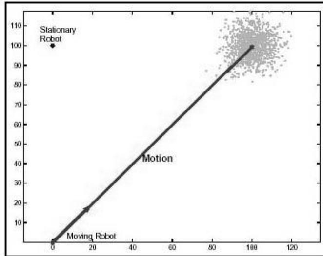
Figure 3.2: The result of prediction (Fox et al. 2000). The robot starts from left-bottom and move to the right-top. Particles on the right-top present the posterior distribution of motion model.
