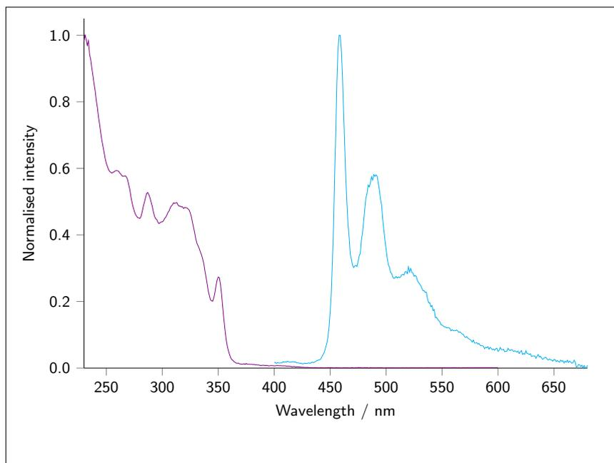
Figure 2.21: Normalised UV-vis absorption spectrum (purple) and emission spectrum (blue) of  $[\text{PtL}^5(\text{ppy})\text{Cl}]^+$  in DCM solution at 298 K.
