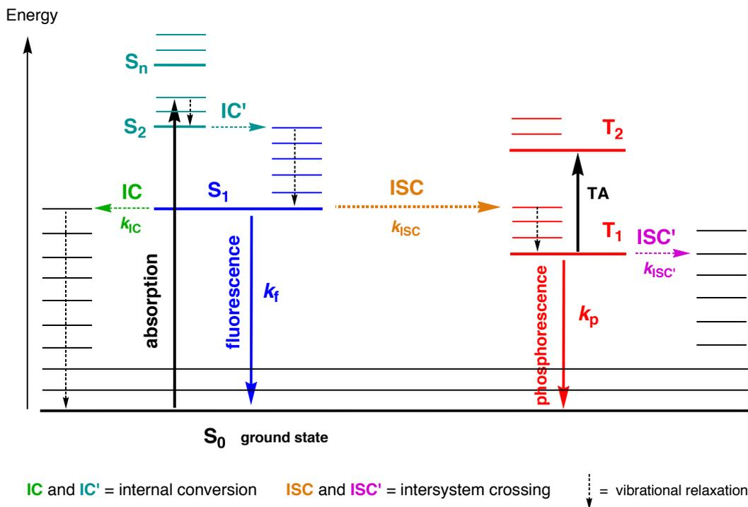
Figure 1.1: A Jablonski diagram to illustrate possible electronic transitions taking place.
