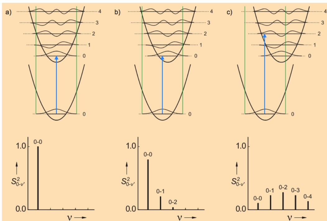
Figure 1.29: Illustration of the quantum mechanical model for Franck-Condon overlap with increasing distortion from a-c.<sup>147</sup>
