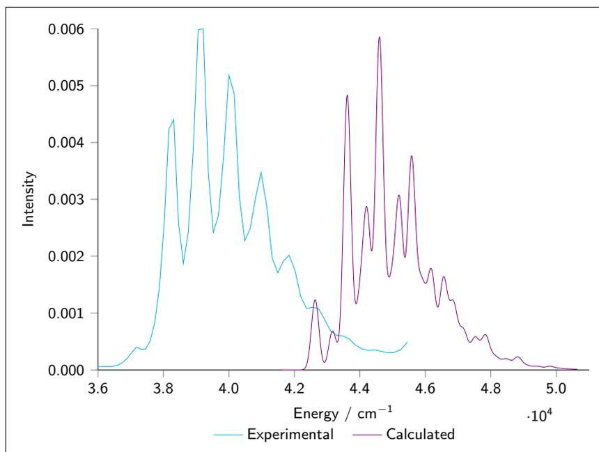
Figure 2.20: Experimental (298 K, in DCM solution) and theoretical (taking into account Franck-Condon factors) absorption spectra of benzene.
