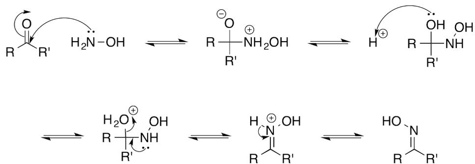
Scheme 5.6: Mechanism for the formation of an oxime.
