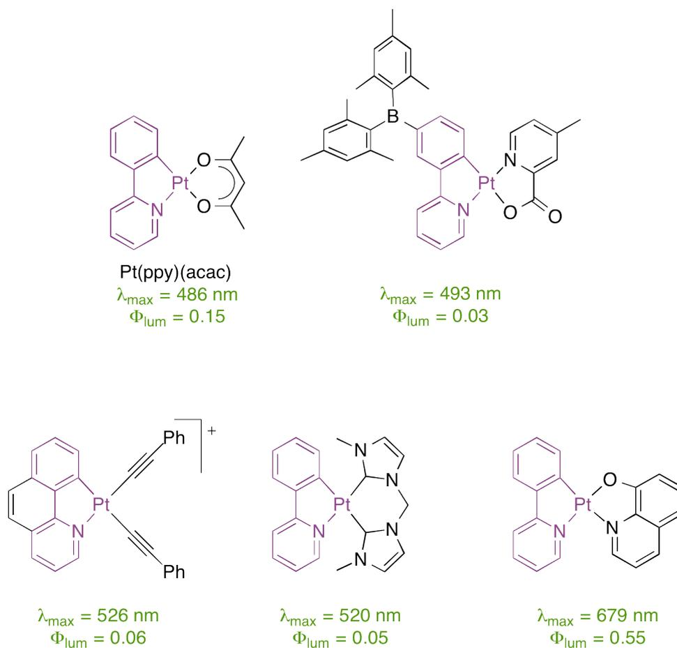
Figure 1.21: Examples of a  $\beta$ -diketonate (top left),<sup>73</sup> 2-picolinate (top right),<sup>82</sup> acetylide (bottom left),<sup>76</sup> carbene (bottom middle)<sup>79</sup> and 8-hydroxyquinoline<sup>83</sup> Pt(II) complex, showing  $\lambda_{\max}$  of emission and  $\Phi_{\text{lum}}$  at 298 K in DCM solution.
