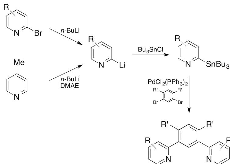
Scheme 2.1: Schematic representation of the ligand formation using Stille cross-coupling.  $R$  represents a methyl group at each of the positions 3-6 around the pyridine ring and  $R'$  represents either a fluorine or hydrogen atom. DMAE = dimethylaminoethanol.
