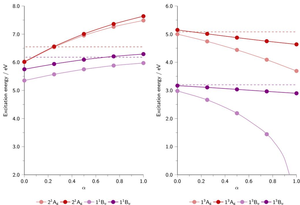
Figure 1.28: Singlet (left) and triplet (right) excitation energies of butadiene as a function of exact exchange ( $\alpha$ ). Dashed lines show reference values.<sup>143</sup> Lighter colours show TD-DFT excitations and darker colours those computed by TDA.<sup>117</sup>
