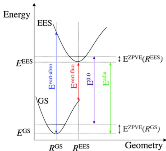
Figure 1.26: Potential energy curve diagram representing two singlet states and possible methods for calculating excitation energies.<sup>100</sup>
