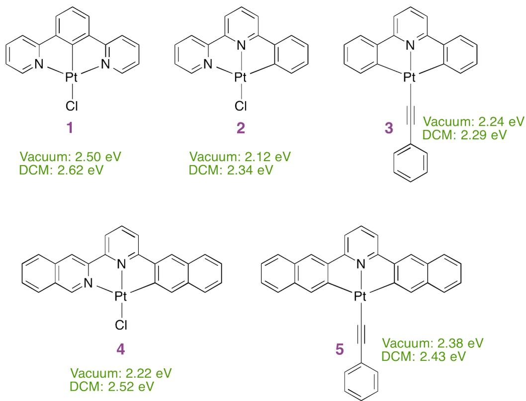
Figure 1.33: Structures and calculated phosphorescence emission energies of the complexes studied by Tong and Che (energies shown for both DCM and vacuum).<sup>154</sup> The  $T_1 \rightarrow S_0$  energies were calculated by the energy difference between the  $T_1$  and  $S_0$  optimised geometries.
