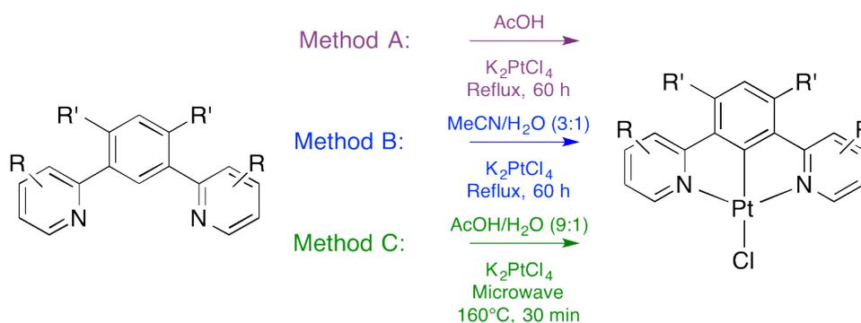
Scheme 2.3: Schematic representation of the three methods used for cyclometallation of the ligand. *R* represents a methyl group at each of the positions 3-6 of the pyridine ring and *R'* represents either a fluorine or hydrogen atom.
