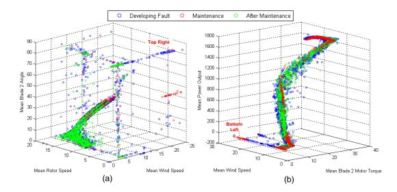
*Figure 3.23: (a) Typical variable-speed pitch-to-feather control plot for Case 1; (b) Pitch torque power curve plot for Case 1;*
