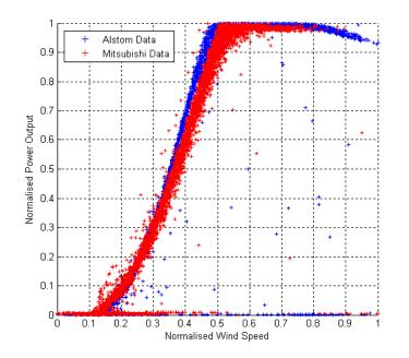
Figure 5.1: Alstom & Mitsubishi WTs, power curve comparison
