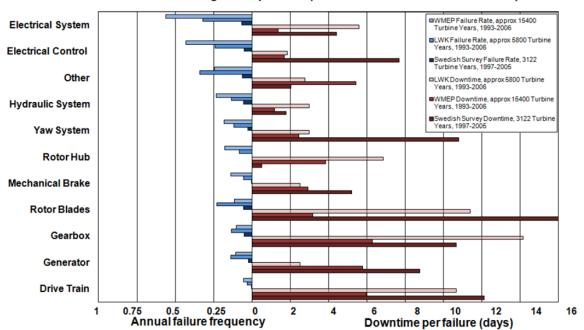
Failure Rate and Downtime from 3 Large Surveys of European Onshore Wind Turbines over 13 years
