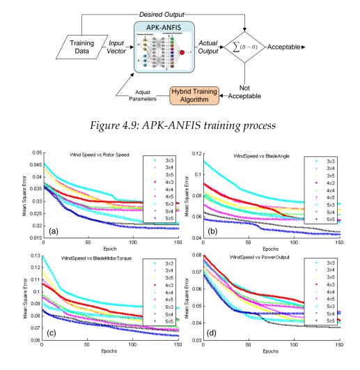
*Figure 4.10: RMSE curve of different ANFIS structures; (a) WindSpeed vs RotorSpeed ANFIS; (b) WindSpeed vs BladeAngle; (c) WindSpeed vs BladeMotorTorque; (d) WindSpeed vs PowerOutput;*
