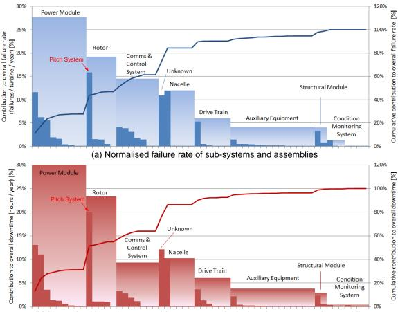
(b) Normalised hours lost per turbine per year to faults in sub-systems and assemblies
