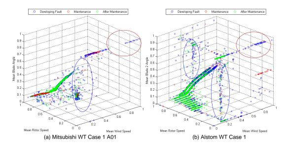
*Figure 5.2: The variable-speed pitch-to-feather/stall plot. Circled in red represent the anomalies, circled in blue represent the noise data.*
