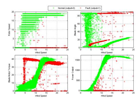
Figure 4.7: Training data from the six known pitch faults.
