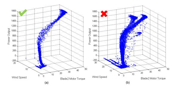
*Figure 3.22: (a) Pitch torque power curve characteristic; (b) An abnormal WT;*
