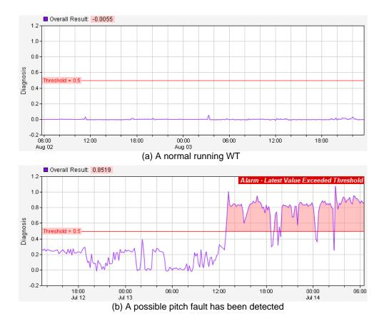
Figure 4.13: Demonstration of the diagnosis system with an arbitrary threshold 0.5
