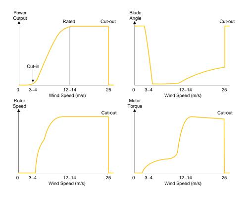
Figure 4.4: Four CCFs for pitch fault analysis
