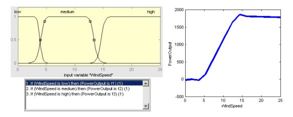
Figure 3.5: The Takagi-Sugeno FIS for WT power output estimation
