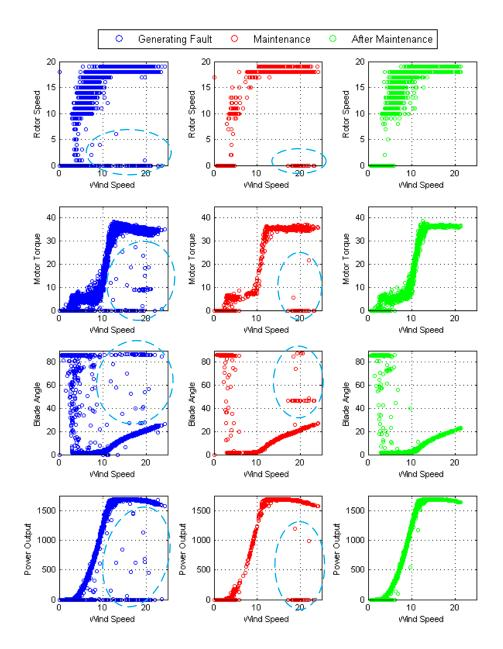
Figure 4.6: Labelling the abnormal data in Case 1
