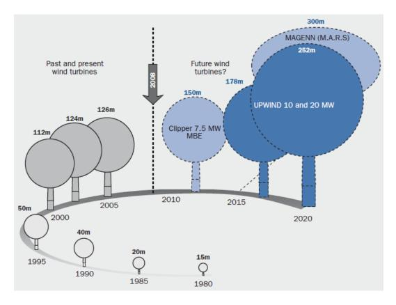
Figure 1.2: Growth in size of wind turbine design (Krohn et al. 2009).
