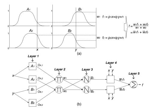
*Figure 4.1: (a)* A two inputs first order Takagi-Sugeno FIS model with two rules; (b) The equivalent ANFIS architecture.
