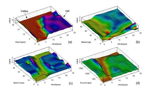
Figure 4.12: Output surfaces generated from the trained APK-ANFIS
