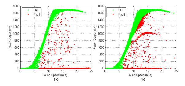
*Figure 3.1: WT power data for investigation purpose (a) Data A; (b) Data B.*
