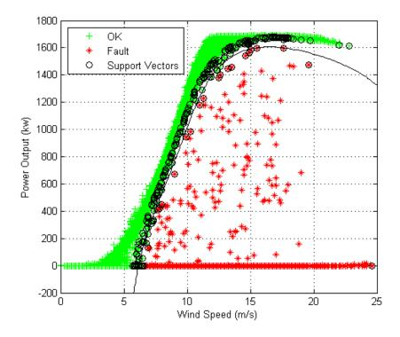
Figure 3.17: SVM result on WT power data A.
