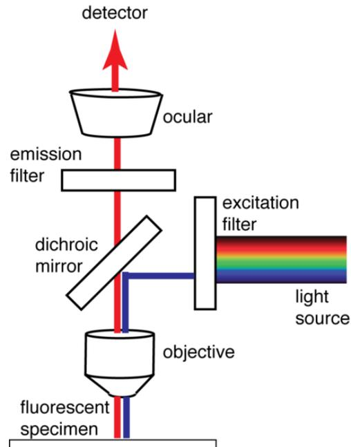
**Fig. 26** Schematic diagram of the typical components of a fluorescence microscope, exemplified by the epifluorescence microscope, where excitation and emission of the sample are both focused by the objective lens.
