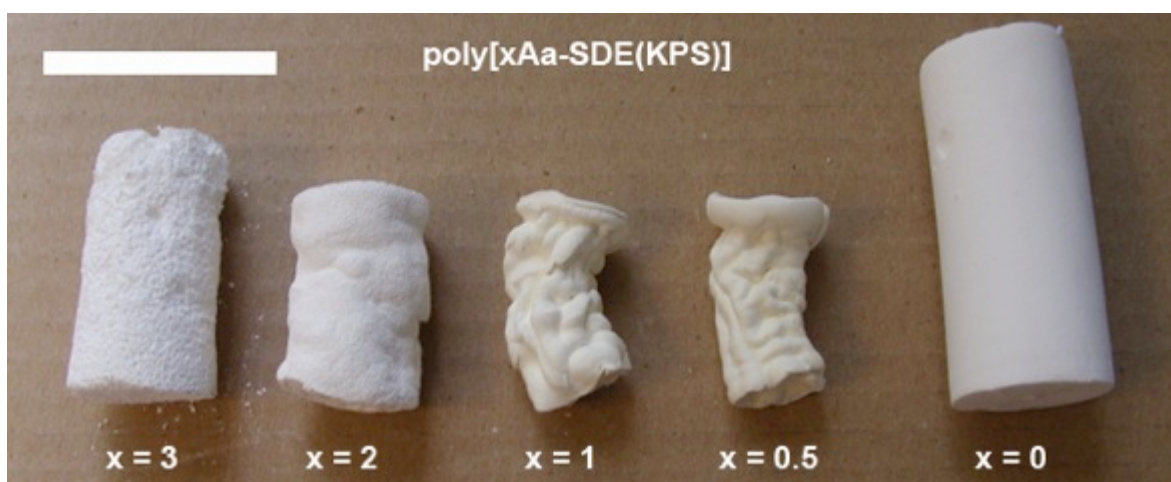
Figure 5.22 Resulting monoliths for low levels of Aa incorporation into polystyrene scaffolds using KPS as the initiator. Even when x < 3 monoliths deform, further demonstrating the unsuitability of KPS as an initiator for Aa incorporation. Scale bar = 4 cm.
