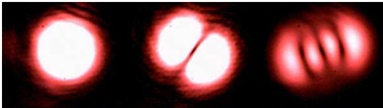
Figure 3.8: TEM_{mn} modes that exist within the high-finesse cavity. Starting from left to right, TEM_{00} (i.e. Gaussian mode), TEM_{01} or TEM_{10} , and TEM_{03} or TEM_{30} .
