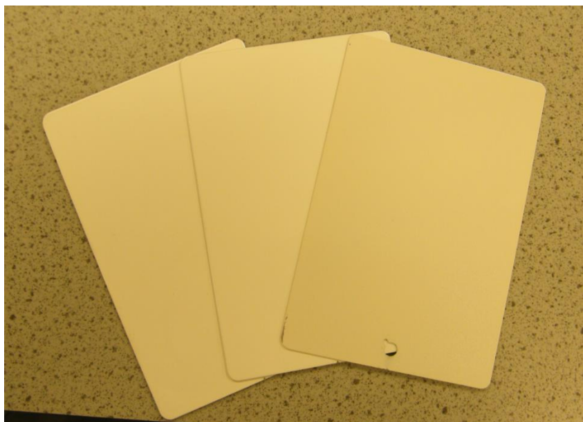
Figure 3.10: Photos of coating samples bound onto Q-panels. From left to right: a current commercial coating (control), and powder coatings derived from 27 ‘H-TMA’ and 28 ‘F-TMA’
