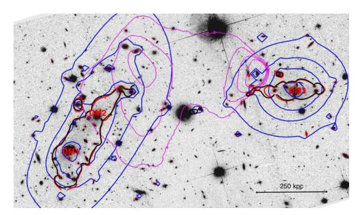
Figure 1.2: Image of the Bullet Cluster from [19]. The blue contours trace the mass distribution, as determined from lensing measurements, while the pink contours follow the distribution of X-ray light. The X-rays trace the distribution of the hot plasma between the clusters. Since the mass is located far from the centre of X-ray emission, this has been taken as evidence for the existence of Dark Matter in this cluster.
