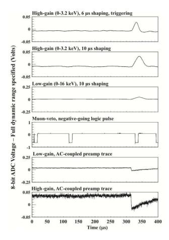
Figure 3.4: An example  $\sim 2.5 \text{ keV}_{ee}$  recoil event in the CoGeNT detector. A recoil induces a sharp change in the measured voltage proportional to the deposited energy. The duration of this rapid change, on the order of a microsecond, is quantified as the rise-time.
