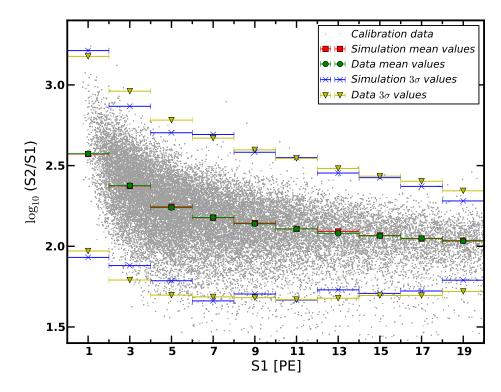
Figure 5.1: Comparison of the mean and spread from our simulated nuclear recoil events with those from the <sup>241</sup>AmBe calibration data. The spread is obtained by fitting gaussian distributions in each S1 bin. The data are only approximately gaussian distributed around the mean and so these  $3\sigma$  values give a good (but not perfect) approximation to the spread of values.
