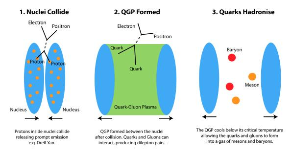
Figure 8.1: Illustration of the formation of the QGP. The nuclei collide, producing prompt emission, such as Drell-Yan, where the protons collide to produce dilepton pairs. After this, a hot plasma of unbound quarks and gluons is formed between the two nuclei, called the quark-gluon plasma. This eventually cools as the nuclei move apart, until the quarks hadronise into baryons and mesons.
