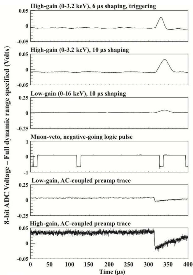
**Figure 3.4:** An example  $\sim 2.5$  keV<sub>ee</sub> recoil event in the CoGeNT detector. A recoil induces a sharp change in the measured voltage proportional to the deposited energy. The duration of this rapid change, on the order of a microsecond, is quantified as the rise-time.
