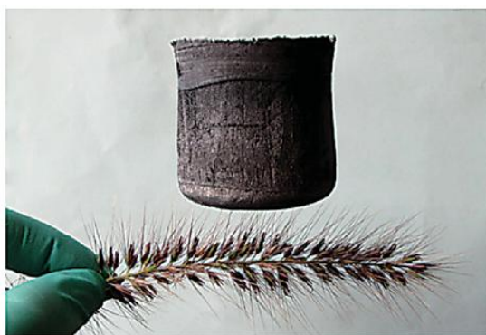
Figure 1.04: A cylinder of carbon aerogel (volume ca. 100 \text{ cm}^3 ) is sufficiently lightweight that it does not deform fine plant fibres. Image reproduced from reference 29.
