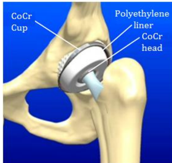
Figure 2.11: Labelled diagram of a dual mobility total hip arthroplasty, modified from video supplied by Biomet.
