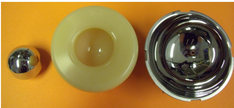
Figure 5.37: 28 mm CoCrMo head, E1 liner, 60 mm CoCrMo cup.
