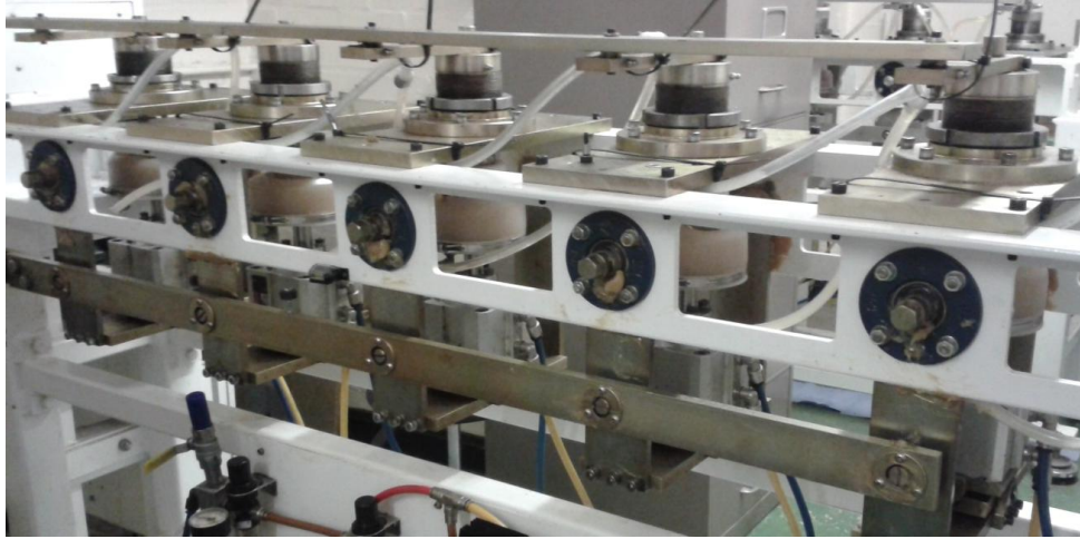
Figure 4.1: Durham hip simulator.
