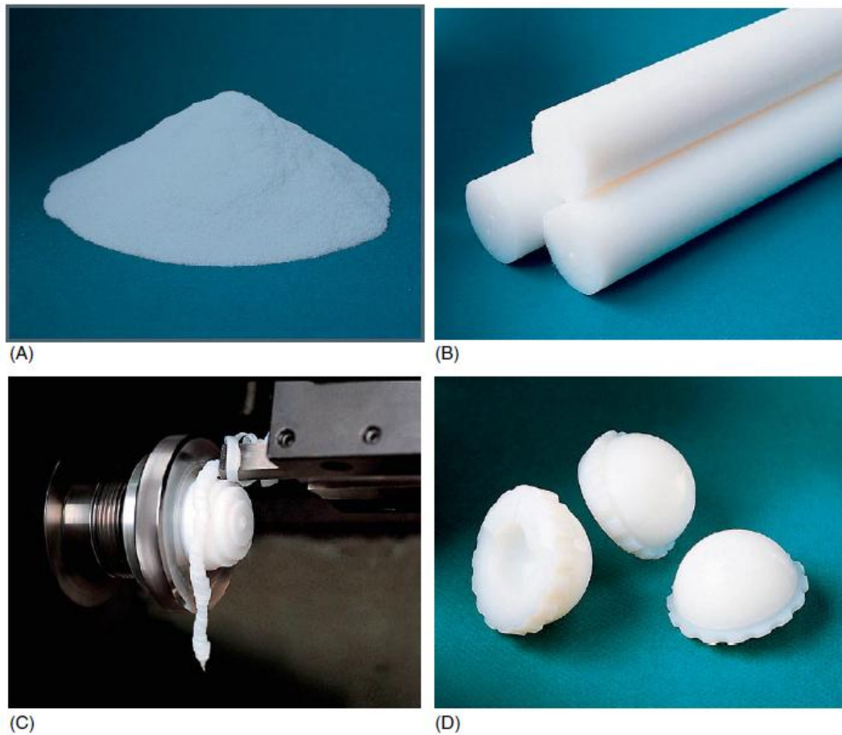
Figure 2.4: Production of UHMWPE acetabular cups. A: UHMWPE resin powder. B: Semi-finished UHMWPE rods that have been consolidated from the resin powder. C: Machining of the UHMWPE rods on a lathe. D: UHMWPE acetabular cups after machining. Images from Kurtz et al. 2009 [30].
