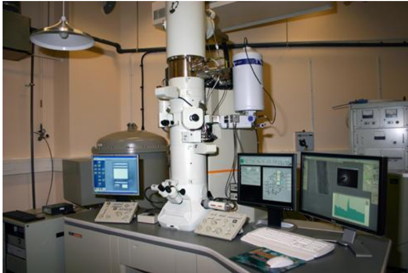
Figure 6.3: JEOL 2100F FEG TEM used in the Physics Dept. of Durham University.
