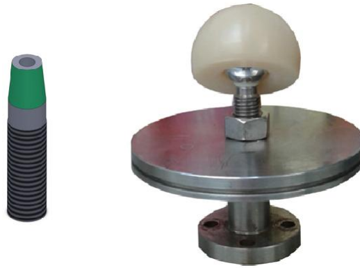
Figure 5.2: Left, PMMA coated stainless steel taper. Right, dual mobility head arrangement held in place with locking nut.
