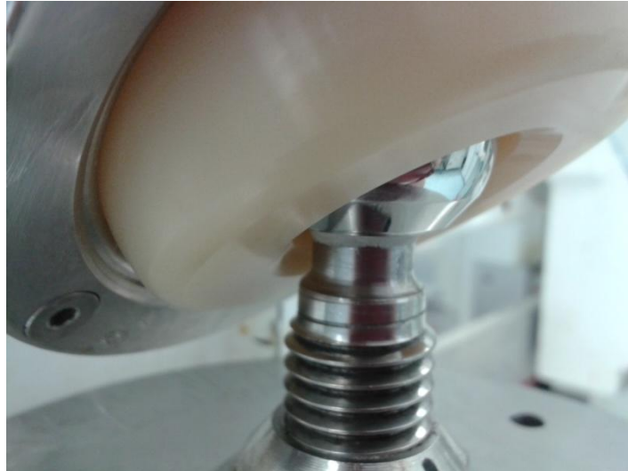
Figure 6.15: Photograph showing the dry set up of the dual mobility joint.
