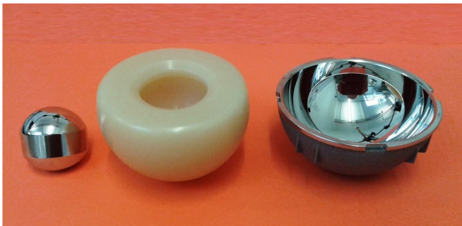
Figure 5.65: 28 mm CoCrMo head, E1 liner, 60 mm CoCrMo cup.
