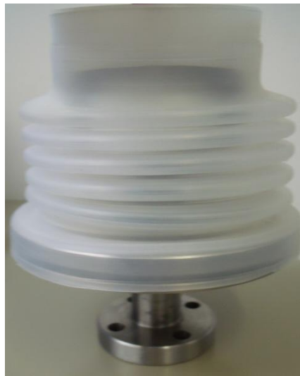
Figure 4.25: Alternative available gaiter with concertinaed edges (pulled over cup holder and base plate).
