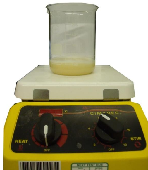
Figure 4.9: HA stirring in test lubricant for 4 hours prior to pin-on-plate simulation.
