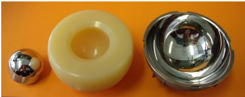
Figure 5.4: 28 mm CoCrMo head, E1 liner, 60 mm CoCrMo cup.
