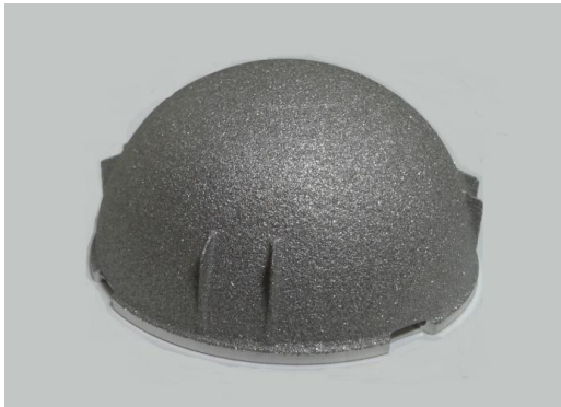
Figure 4.4: Porous titanium coating on the back of CoCrMo acetabular cup.
