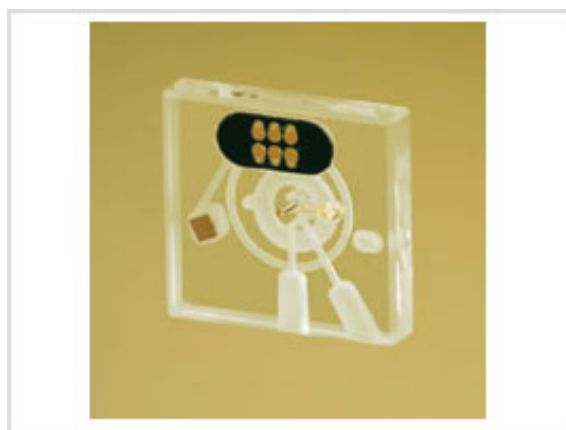
Figure 2.7: A Photograph of the MTFML flow cell. Courtesy of Bruker Corporation.
