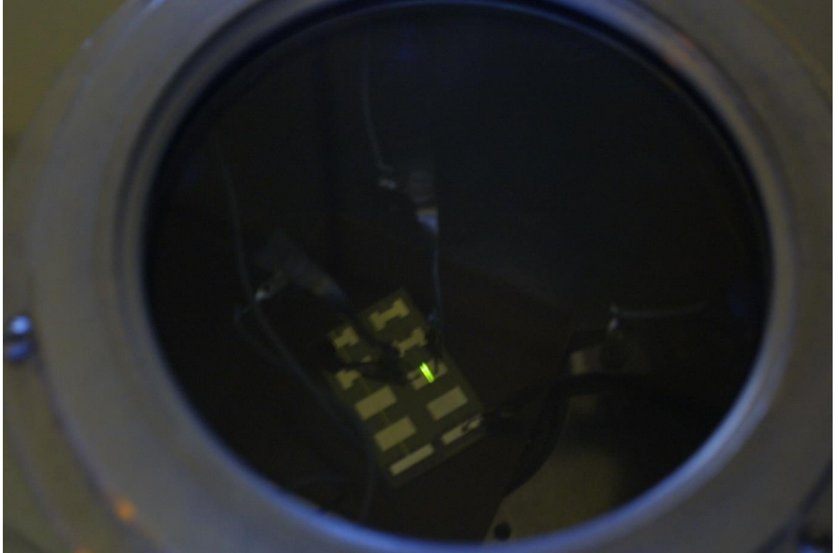
Figure 8.22: Photograph of a transistor device emitting light. Channel dimensions: L = 50 \mu\text{m} and W = 4000 \mu\text{m} .
