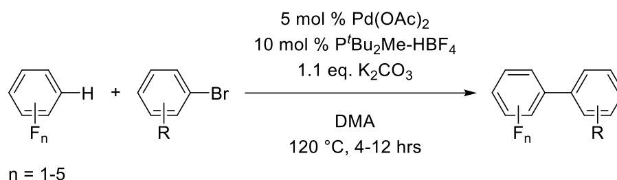
Scheme 26. Catalytic intermolecular direct arylation of polyfluorobenzenes. 103
