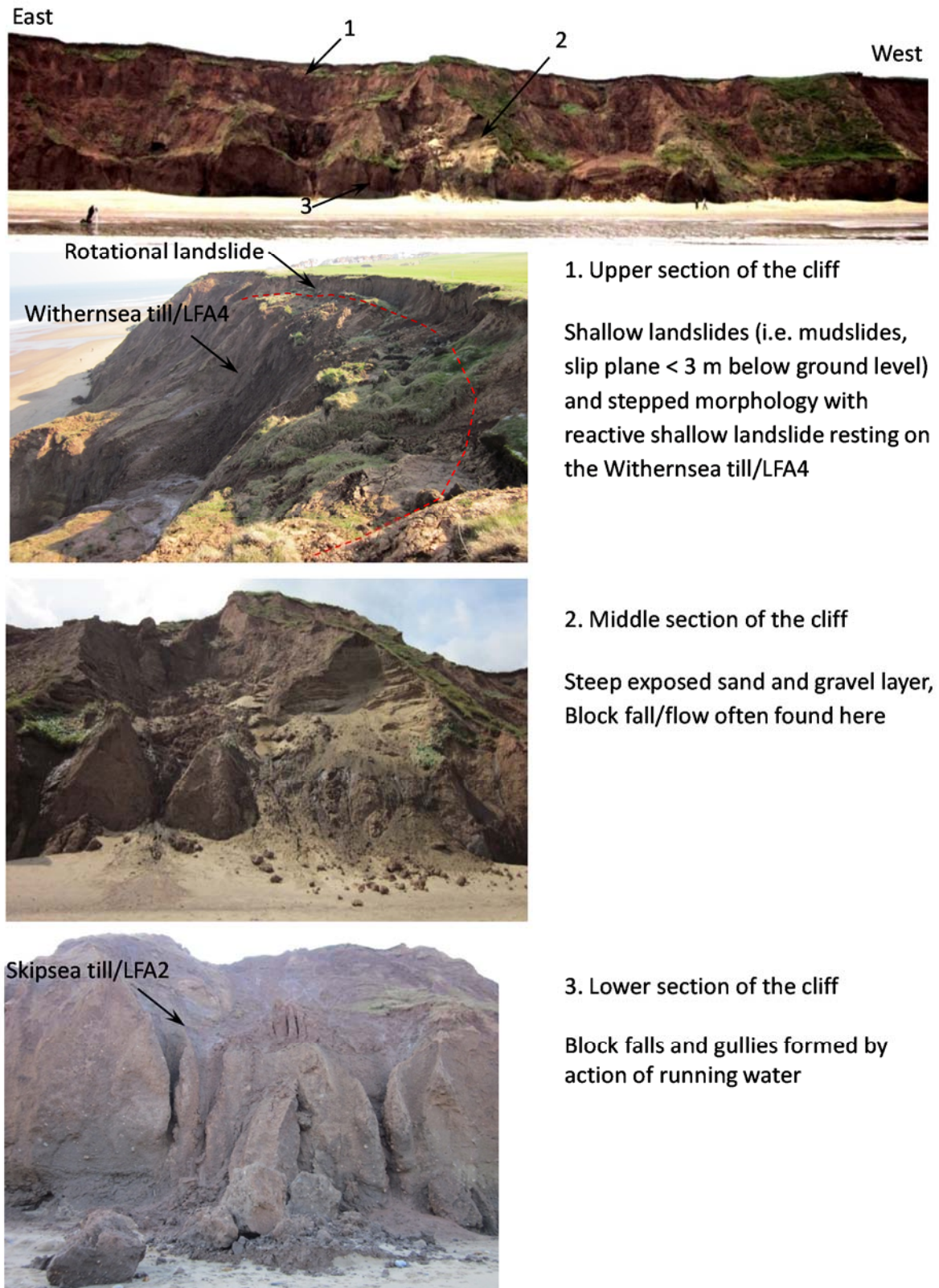
Figure 3.3 Characteristics of glacial till at the Upgang cliff and landslide features of the upper section (1), middle section (2) and lower section of the cliff (3)
