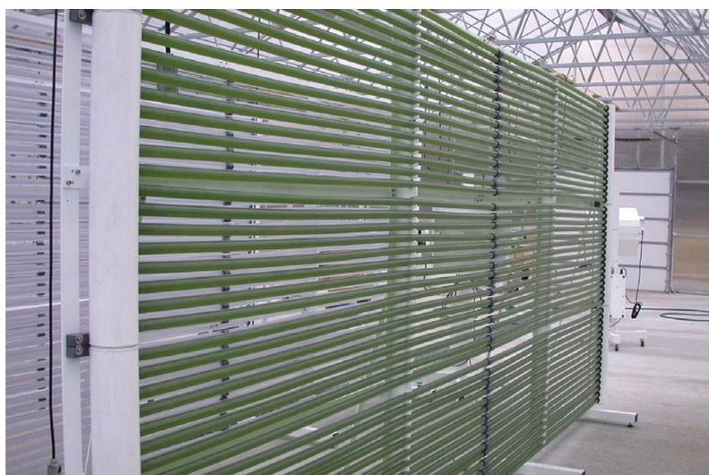
**Figure 1.4 Tubular photobioreactor for algae production. Taken from Greenwell *et al.*<sup>51</sup>**
