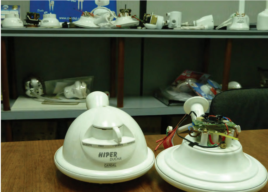
Figure 5.9: Components of an electric shower.
