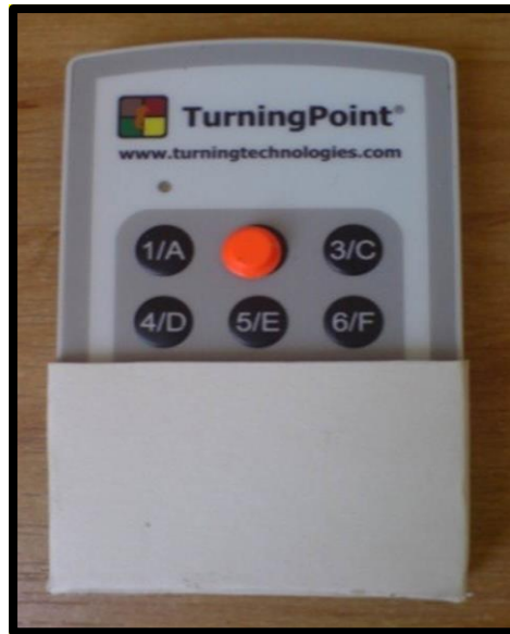
Figure 38. Keypad adapted with orange bumpon and cover for data collection from BPSPs
