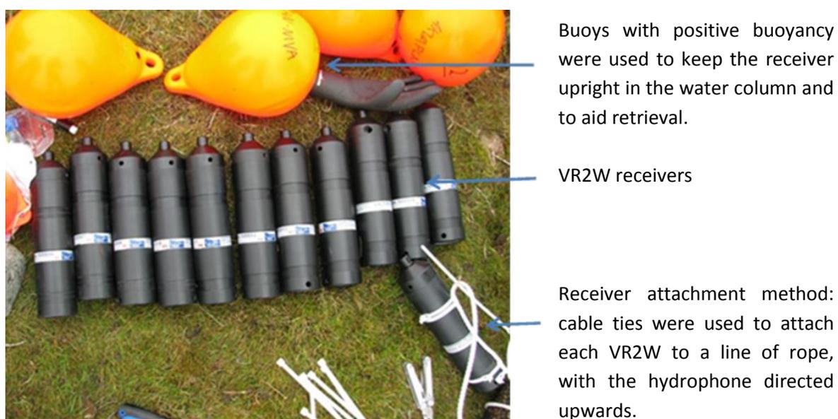
Figure 4-5: Receivers used for VPS deployment in Lake Ellasjøen, Bear Island. The figure also illustrates the attachment method used for receiver deployment.
