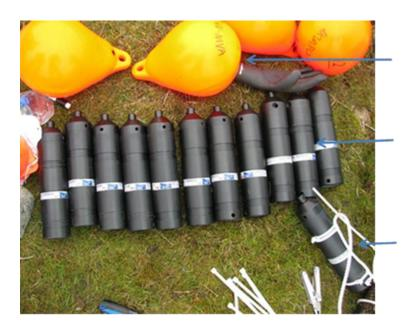
Buoys with positive buoyancy were used to keep the receiver upright in the water column and to aid retrieval.
