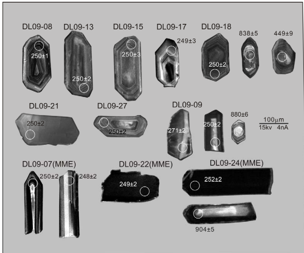
Fig. 3.6. Cathodoluminescence (CL) images of zircons from representative samples. White circles are the analyzed spots. The values with error are ages in Ma.
