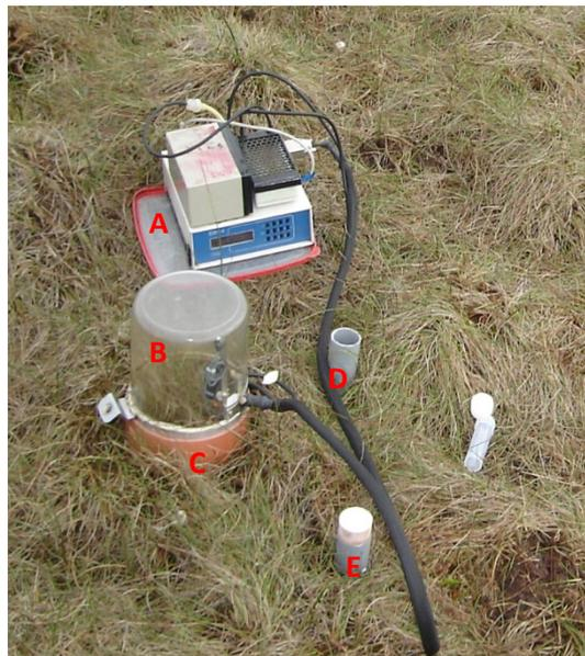
Figure 2.4 Experimental plot set-up: A = infra-red gas analyser; B = chamber; C = gas collar; D = dipwell; E = surface water runoff trap
