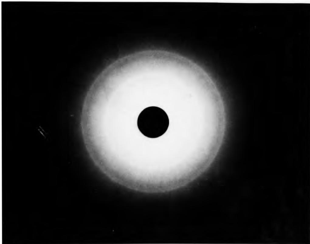
Fig.A.9(b) X-ray Back Reflection - CdSe after Heating
