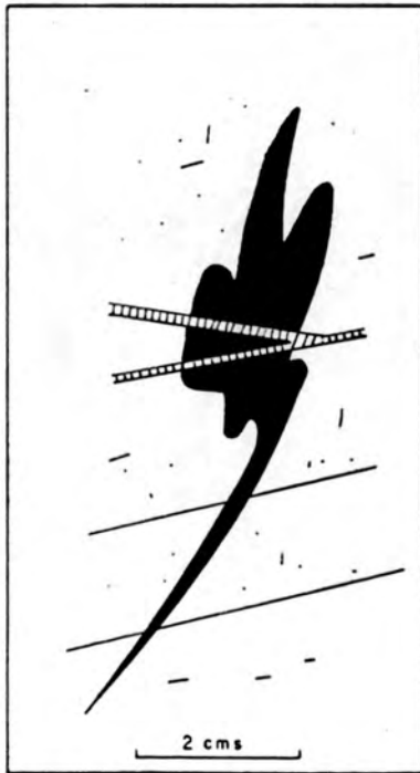
Figure 5. Inclusion of chrome ore in dunite, Kalung Islands. Contacts are sharp. Note streaks and tails of ore.
