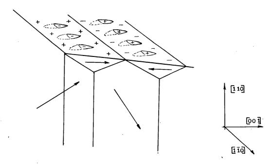
Fig. 11. Possible domain arrangement in a strained crystal.
