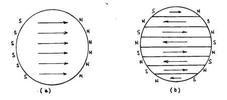
Fig. 1. Sphere of iron, (a) magnetised uniformly and (b) divided into domains.
