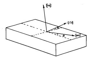
Fig. 4. Orientation of specimen face.
