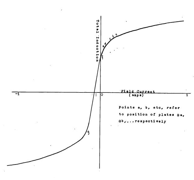
Fig. 15. Variation of magnetic induction with field current.
