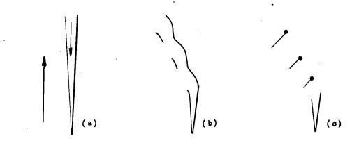
Fig. 14. Reverse dagger (a) becomes stepped dagger (b) then steps close to form tadpoles as in (c).
