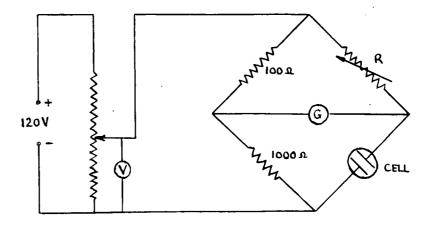
shown in fig 7. For various applied voltages, measured on V, the resistance R was adjusted to give zero deflection on the galvanometer G. The cell resistance was then 10 x R and a maximum cell
