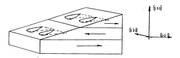
Fig 13 Formation of daggers on face inclined to a.(110) plane
