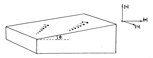
Fig 16 Tadpoles on face inclined to a (110) plane
