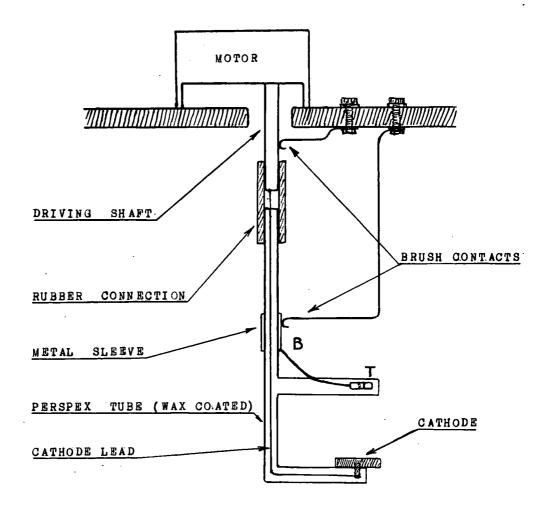
Fig 5 Polishing apparatus
