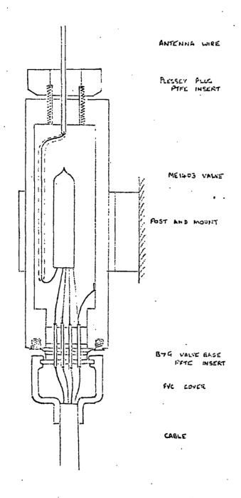
Fig. 11. Experimental Valve Housing after Spangler
