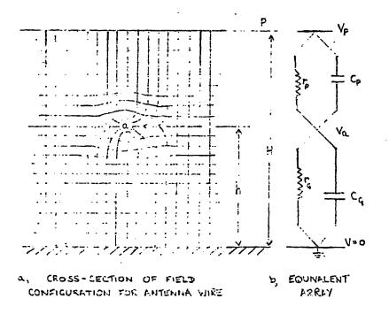
Fig. 8. Passive Probe Equivalent Circuit
