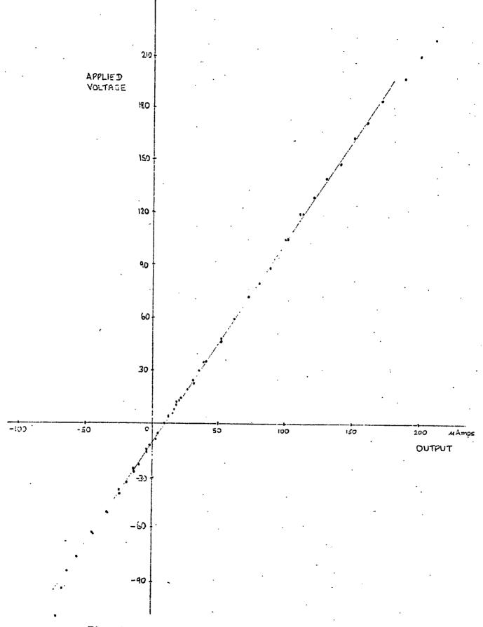
Fig. 12. Calibration Curve of Passive Probe
