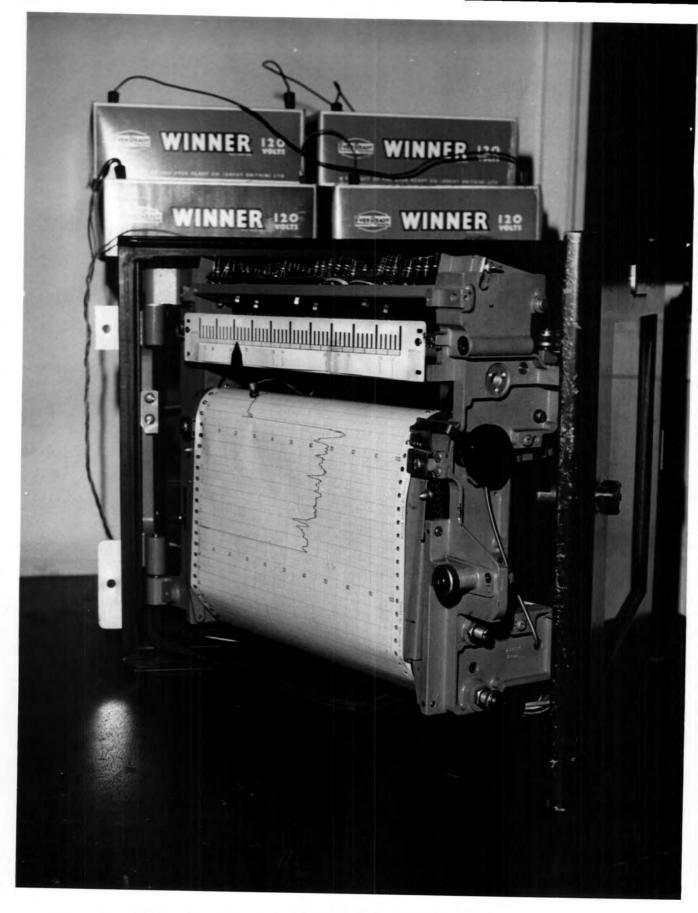
Plate 4 The Potential Balancing Servo Mechanism
