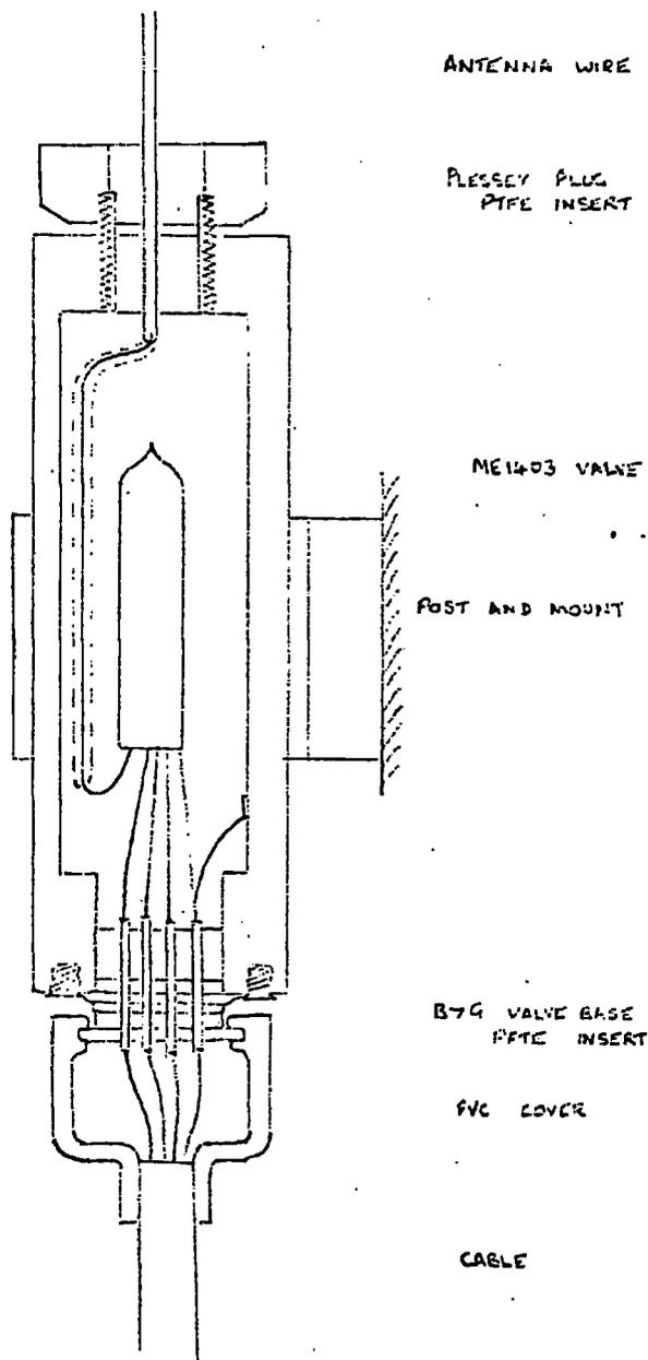
Fig. 11. Experimental Valve Housing after Spangler
