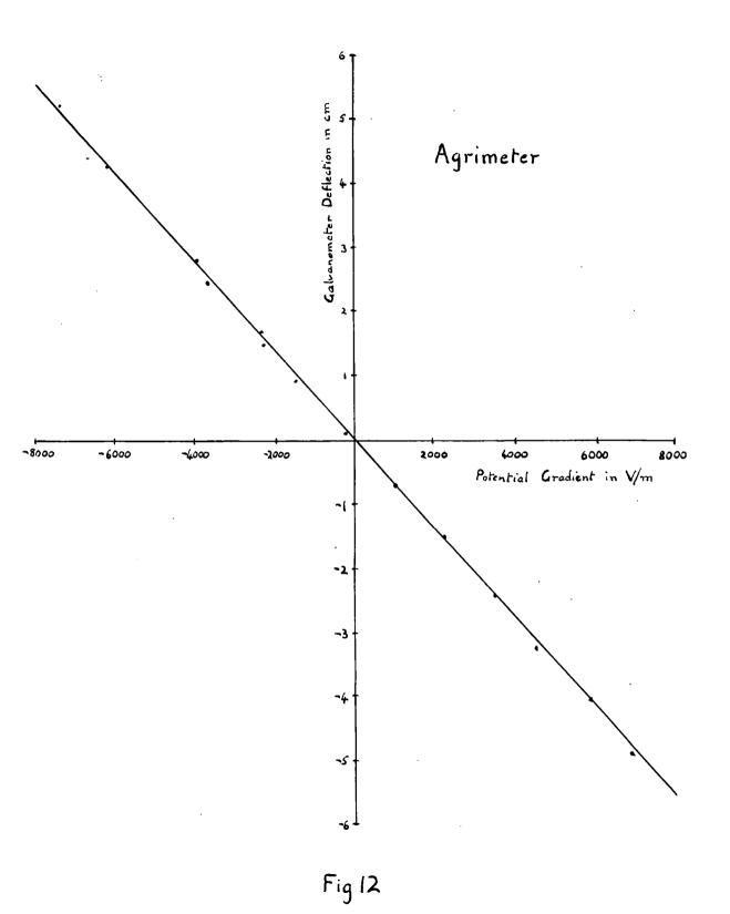
the relation could be found between the potential gradients thus produced and the outputs of the instruments (Figs. 11 and 12).
