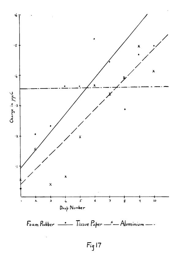
splashing the rest struck a surface consisting largely of water and splashed badly (Fig. 17). Padding of this type would have reduced the current due to splashing on the edge in light rain, but would have become waterlogged rapidly in heavier rain and lost its effectiveness. An ideal material would have been one that was soft enough to prevent splashing and was also sufficiently porous to provide good drainage in order to avoid the accumulation of water on its surface.
