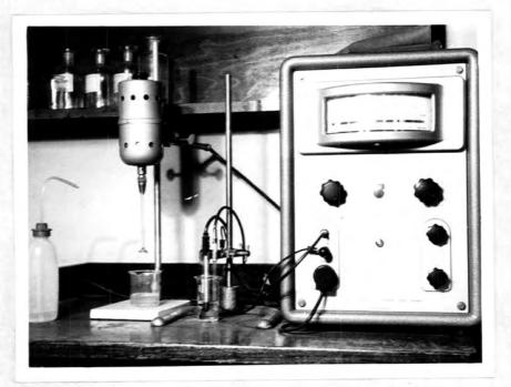
PLATE 10. E.I.L.pH Meter and mechanical stirrer.
