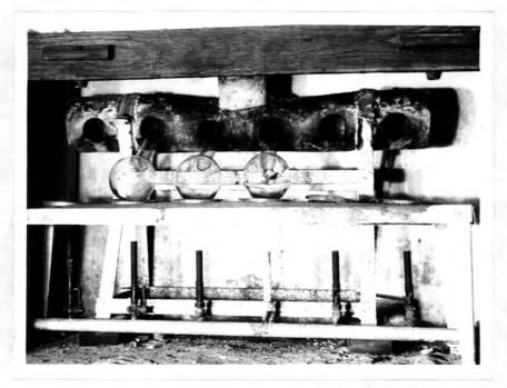
PLATE 8. Digestion apparatus for nitrogen determination.
