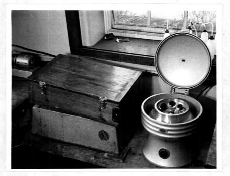
PLATE 11. Mechanical shaker and centrifuge apparatus.
