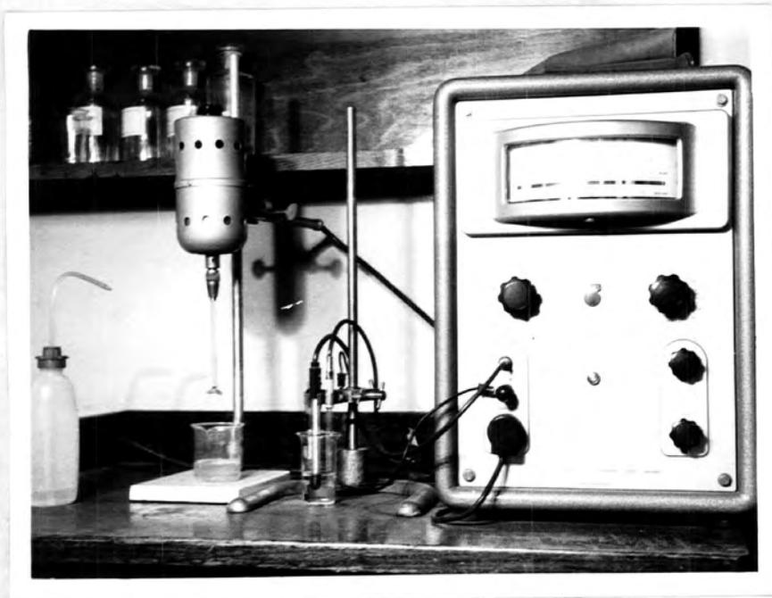
PLATE 10. E.I.L.pH Meter and mechanical stirrer.
