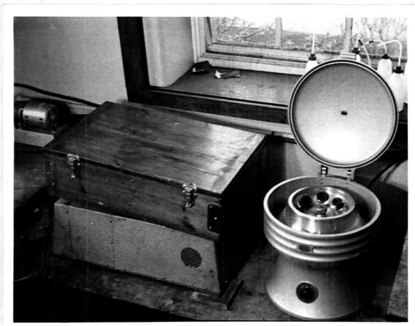
PLATE 11. Mechanical shaker and centrifuge apparatus.
