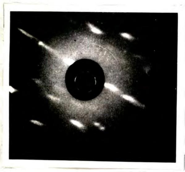
Plate 61. Laue back-reflection photographs of a highly stretched silver single crystal. (After Andrade, 1950).
