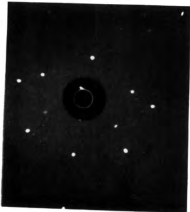
Plate 64. Fine beam of X-rays reflected back from a single crystal of gold. (After Andrade, 1956).
