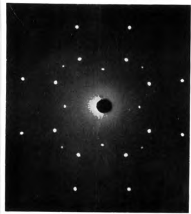
Plate 62. Fine beam of X-rays passing through a crystal of cubic structure. (After Andrade, 1956).
