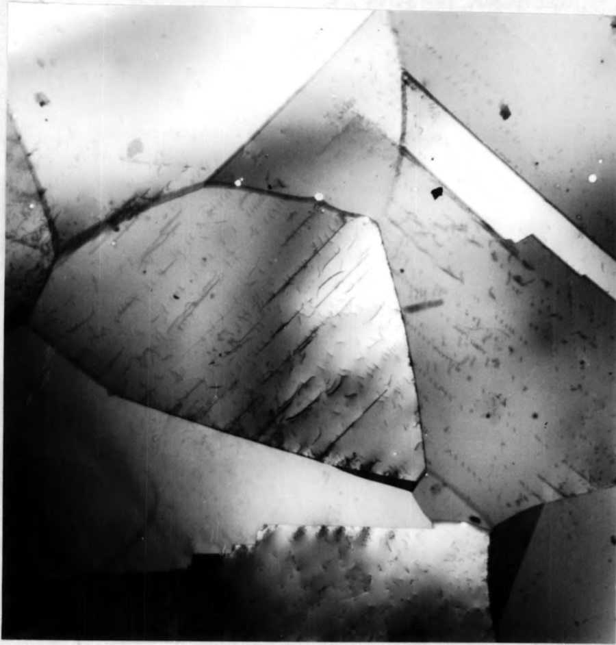
Plate 44. Pile ups in a lightly rolled specimen of stainless steel. ( x 3340) (After Whelan, Hirsch, Horne, and Bolliman, 1957).
