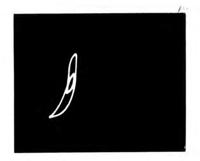
1/2 sub-harmonic with Stalloy cored reactor (120 turns C.T.)
