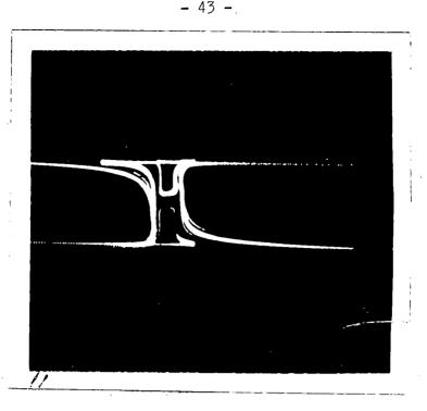
Hysteresis Loop of long persistence (1 - 2 minutes) <sup>1</sup>/4 sub-harmonic Scales B =  $1.5 \text{ Wb/m}^2/\text{cm}$ . V = 85 volts. C =  $160 \mu$  F  $I_s = 0.15 \text{ A/cm}$ . C' = 50  $\mu$  F.
