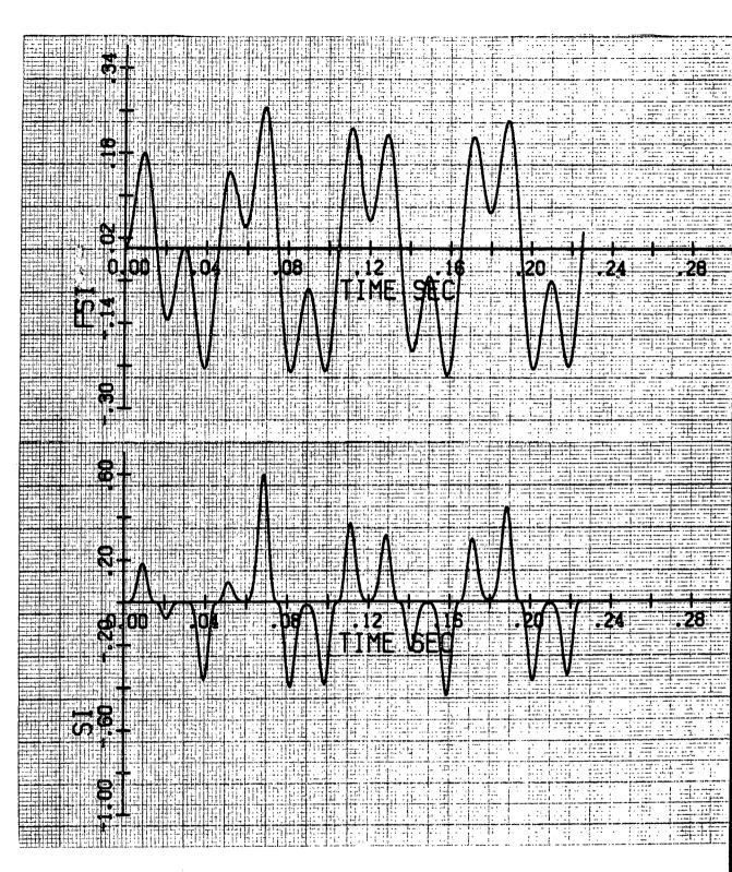
Computer drawn curves for digital solution of Duffings equation, equation 8, showing  $\frac{1}{3}$  sub-harmonic response after the initial transient period.
