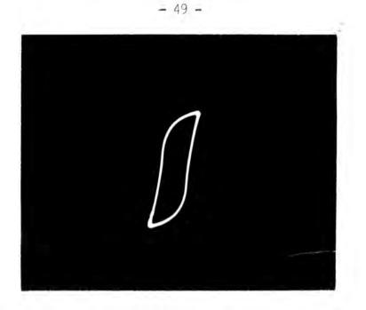
. Normal Hysteresis Loop of Stalloy (120 turns C.T.) core. Scales  $B = 1.0 \text{ Wb/m}^2/\text{cm}$ .
