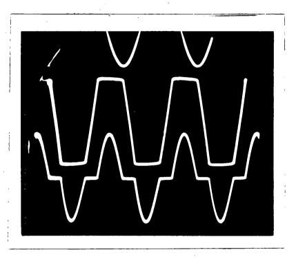
Saturable reactor flux and current during fault current
