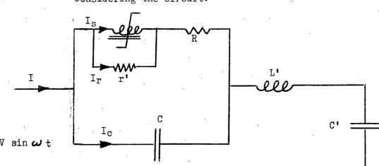
where r' represents the reflected damping resistor r. Neglecting the voltage drop across L' compared to the voltage drop across C'.
