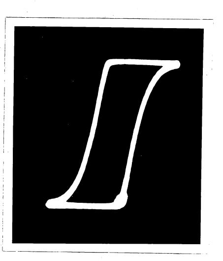
Normal Hysteresis Loop of H.C.R. Alloy core with 50 Hz sinusoidal excitation on 250 turn winding.
