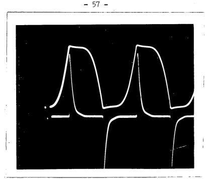
. Saturable Reactor Flux and current waveforms of ferro-resonance phenomena during fault current limitation.
