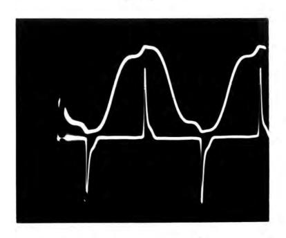
Saturable reactor flux and current during  $^{1}/_{3}$  sub-harmonic response.
