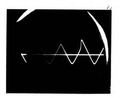
Hysteresis Loop and waveform of charge on the capacitor for a series circuit exhibiting 1/2 sub-harmonic response.
