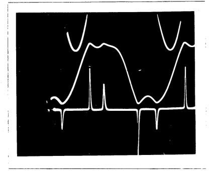
Saturable Reactor flux and current waveforms of ferro-resonance phenomena during fault limitation, but with gross detuning of the link. Scales B =  $1.0 \text{ Wb/m}^2/\text{cm}$ . Conditions V = 100 volts.  $I_s = 4 \text{ A/cm}$ . C = 80 // F.
