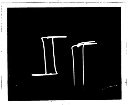
Hysteresis Loop for sub-harmonic response showing details of minor loop.
