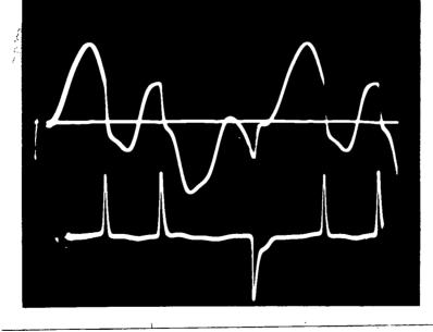
Capacitor/Saturable Reactor Voltage during  $^{1}/_{3}$  sub-harmonic response.
