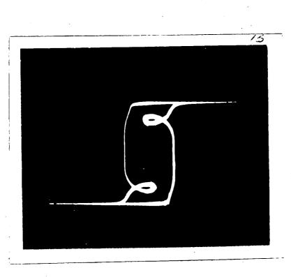
Hysteresis Loop with r = 31 ohms on 50 turn winding. <sup>1</sup>/3 sub-harmonic response just about to extinguish. Scale  $B = 0.76 \text{ Wb/m}^2/\text{cm}$ . V = 100 volts.  $I_s = 0.11 \text{ A/cm}$ .  $C' = 23 \mu F$ .
