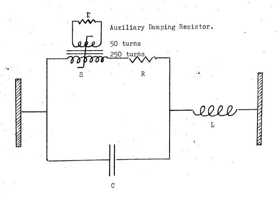
Connection of Auxiliary Damping Resistor 'r' to quench the sub-harmonic response.
