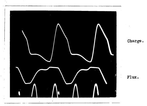
Waves of capacitor charge and saturable reactor flux for the series circuit with 1/2 sub-harmonic response. Both charge and flux show 1/2 sub-harmonic. This is the trapped charge of Travis' paper.
