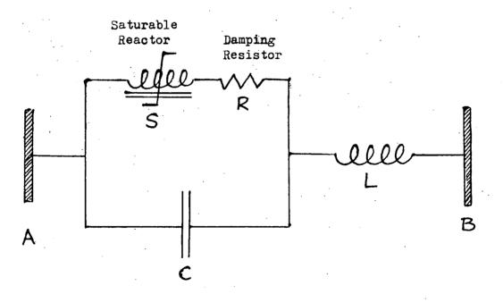
d) Alternative proposed method of limiting the voltage across the capacitor and hence destroying the resonance state under fault conditions.
