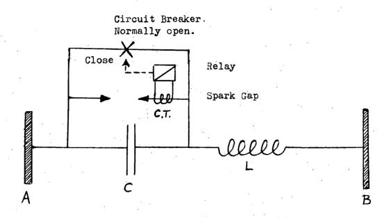
c) Resonant link designed to short circuit the capacitor under fault conditions. see ref.12 E. Friedlander.
