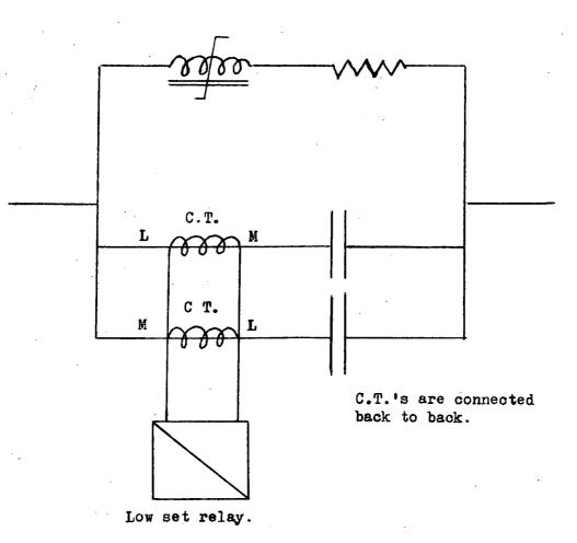
such a system would detect any imbalance in the capacitor branches.
