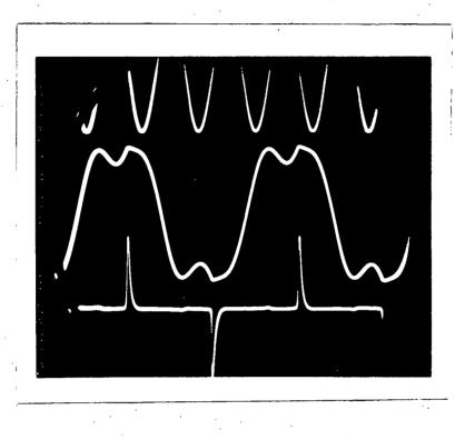
$^{1}/_{3}$  Sub-harmonic with a resistive load of 550 ohms with an applied voltage of 180 volts. R.M.S. Scales B =  $1.0 \text{ Wb/m}^{2}/\text{cm}$ .  $I_{s} = 1.0 \text{ A/cm}$ .
