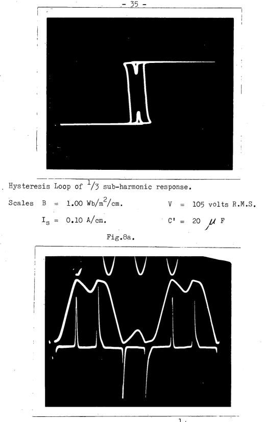
Saturable reactor flux and current during 1/3 sub-harmonic response.  $C' = 20 \mu F$ . V = 105 volts. R.M.S.
