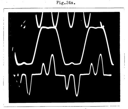
Saturable reactor flux and current during 1/3 sub-harmonic response. Scales B = 1.0 Wb/m<sup>2</sup>/cm. Conditions V = 100 volts.
