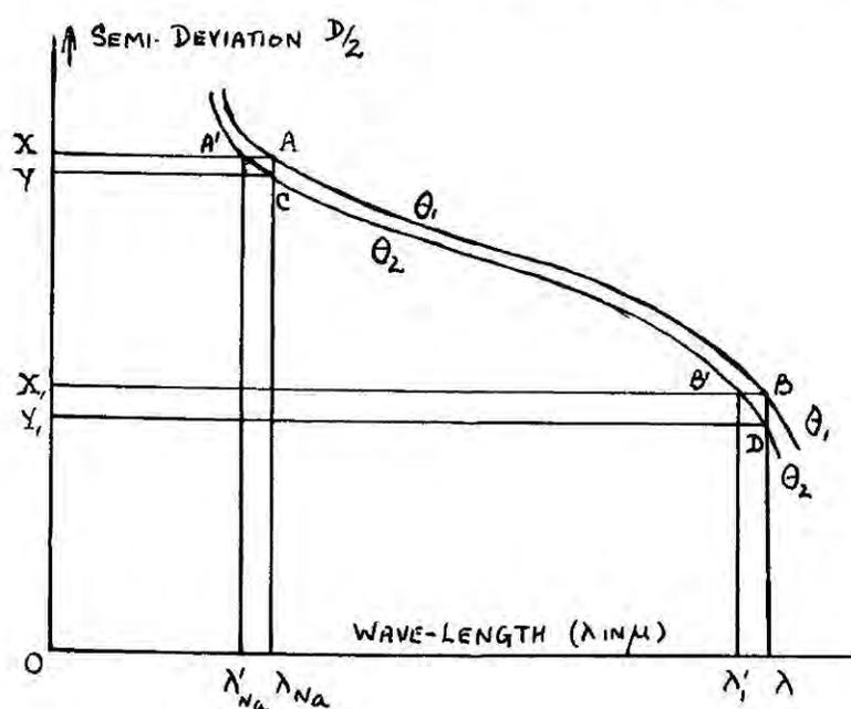
is  $\lambda_{Na}$ ; and similarly, a difference will be noticed at other wave-lengths: for a drum setting of  $\lambda_1$ , the wave-length transmitted by the thermopile slit will be  $\lambda'_1$ .
