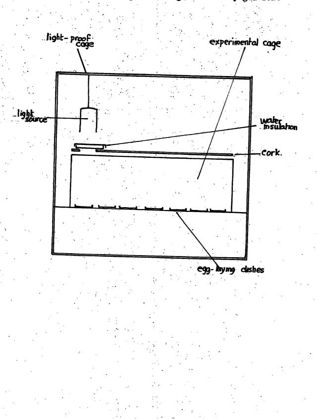
Apparatus used to produce light-intensity gradient
